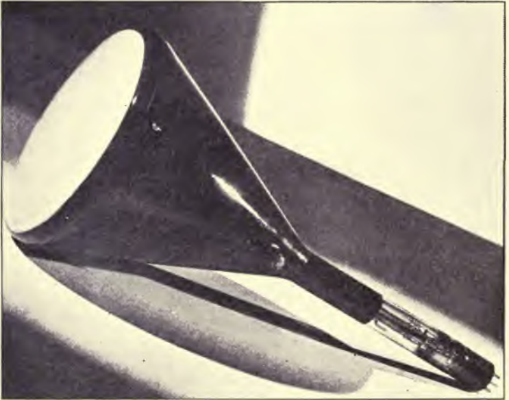
FIG. 51—The heart of the television receiver is the kinescope or picture tube, two types are illustrated.
