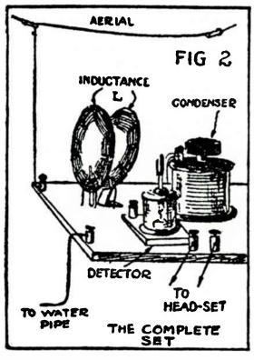
Such a condenser could not be made without the use of a good set of tools, and the author strongly advises it be bought instead of made at home in order to avoid trouble. The aluminum plates are spaced very closely and great care should be taken to avoid bending them, as they must not touch each other.
