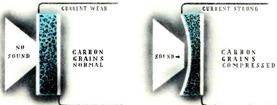
the wires depend entirely upon the vibrations of this metal plate. This device makes the telephone transmitter or the radio microphone work. You might have seen the little compartment if you have ever unscrewed the transmitter end of your phone.
