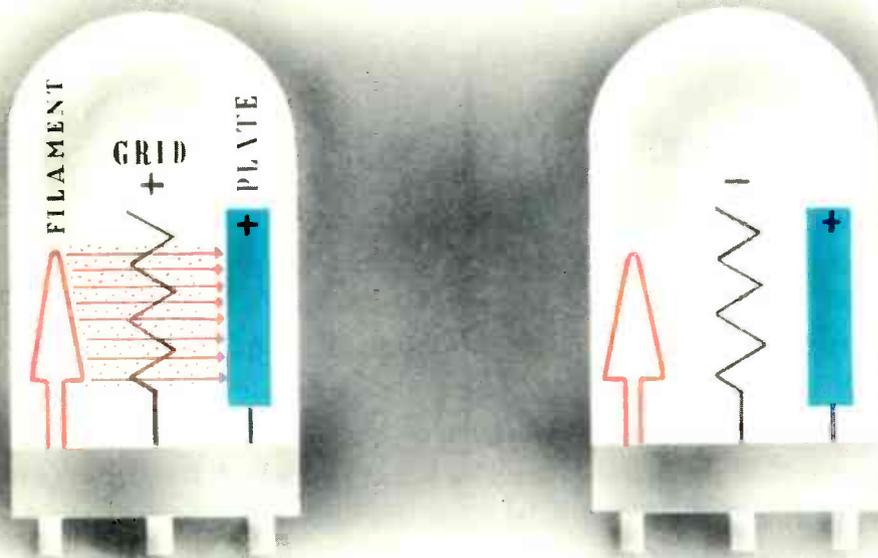
vacuum tube we have three things: a hot glowing filament, a tiny wire grid that is charged with the alternating current of the incoming radio waves, and a small metal plate that is always charged positively.
