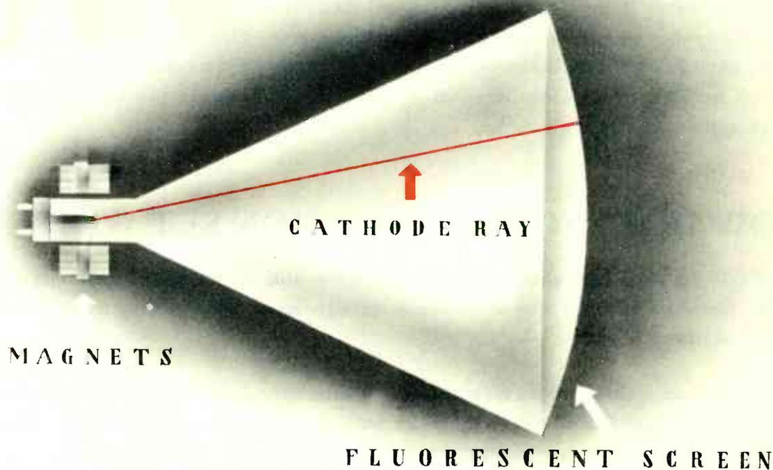
The electromagnets in your set also control a cathode-ray beam. This beam moves inside the kinescope and covers your television screen in the same way that the
