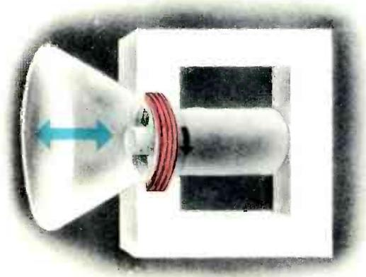
**T**HIS thin iron disc close to an electromagnet is the principle on which the receiver of your telephone or the loud speaker of your radio set works. You might have seen this disc and electromagnet if you have ever unscrewed the receiver end of your phone. In your loud speaker the metal disc is attached to a large cone made of strong paper, and the vibrating paper cone gives you the sound.
