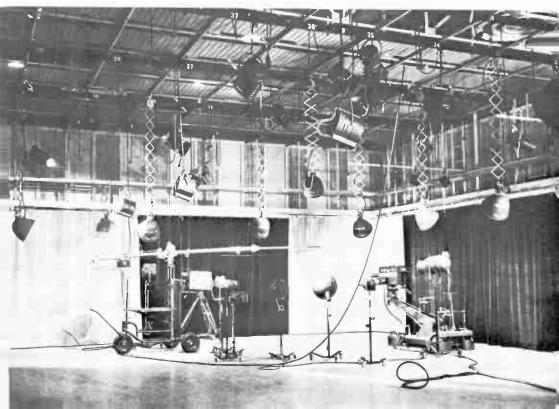
performers or objects, may be floor banks or single-unit scoops or fresnels. Fixed or focusing spots are used for *highlighting*; that is, bringing some object in the picture into special prominence. Crossed spots can highlight a merchandising display and at the same time counteract each other's shadows.
