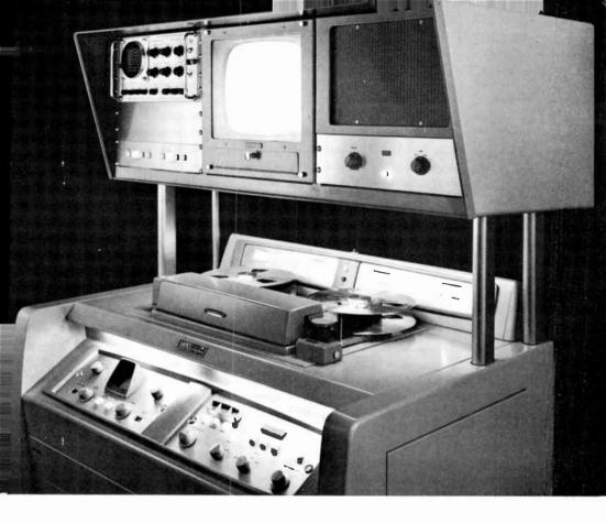
Figure 59. Videotape, Ampex VR-1000 Magnetic Recorder.
