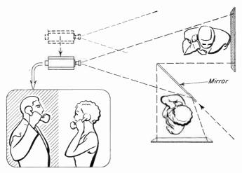
Fig. 11-9. Split-screen effect done by a mirror. Dash arrows indicate two methods of wiping in the reflected image: trucking the camera and sliding the mirror.
