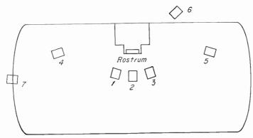
Fig. 20-36. Diagram of camera positions used in pool coverage at the 1960 Democratic convention. 1, 2, and 3: basic front shots. 4 and 5: side angles. 6: high-angle over-the-shoulder position. 7: high-angle end view for wide-angle establishing shot.
