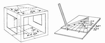
Fig. 5-21. Bretz box, with method of laying out windows.
