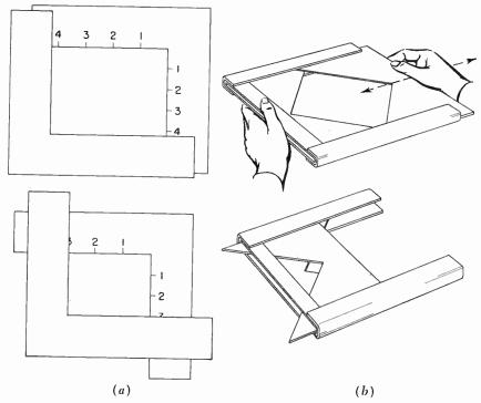
Fig. 9-24. L-shaped framing guides. Bretziframe sliding framing guide. Retains 3 by 4 aspect ratio.
