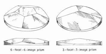
Fig. 11-21. Two types of multiple-image prisms.
