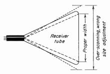
Fig. 8-6. When the height and width controls on a receiver are set for too wide a sweep, the beam will strike the sides of the tube and only the center of the broadcast picture will be seen.
