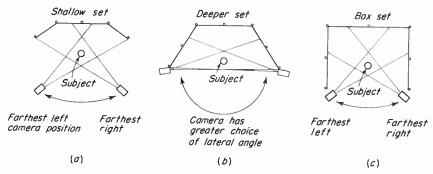
Fig. 16-14. What shape and depth should a simple set have for best choice of camera angles? (a) Shallow set limits use of cameras for side angles. If they go too far to the side, they will shoot off set. (b) Deeper set allows greater freedom in use of side angles. (c) Box set with walls at right angles to back again prevents cameras from moving to the side (unless they go into the set).
