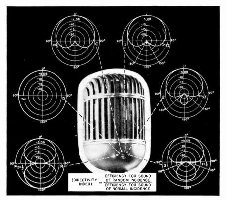
Fig. 19–12. Western Electric Cardioid microphone, showing variety of directional patterns.
