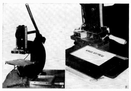
Fig. 9-23. Kensol hot-press machine. Standard lead type is locked into chase at right which is attached to head, heated, and brought down onto the card by manual pressure. Opaque roll leaf is laid on top of card and pressed in by the type.
