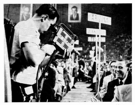
Fig. 3-4. Vidicon "R-F" or wireless camera which does not require a cable. (R-F: radio frequency.)
