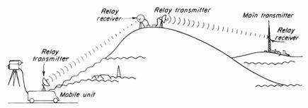
Fig. 20-7. Double jump is used when line of sight is obstructed.
