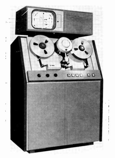
Fig. 23-9. The Ampex VR 8000. The single head rotates inside the drum at center as the tape moves around it in a helical wind.
