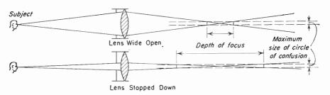
Fig. 5-27. Why depth of focus is improved by stopping down the lens.
