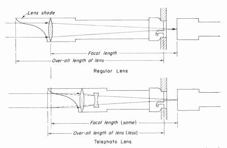
Fig. 5–23. Comparison of regular lens with telephoto lens of the same focal length. Both produce the same picture.
