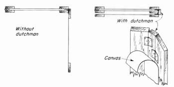
Fig. 16-6. Method of constructing a threefold flat so that it can be folded flat. The wooden dutchman is inserted between two of the flats.
