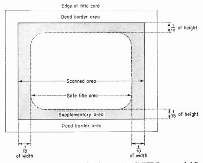
Fig. 8-8. Method of determining safe title area. From SMPTE Recommended Practice (RP8), established May 7, 1961.
