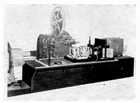
Fig. 10-4. RCA multiplexer with cover removed, showing cube prisms. Slide projector at left projects through both prisms. Film projector at back is reflected by inner surface of left-hand cube. Right-hand cube provides for another projector position on near side. A 45-degree mirror between the field lens and the camera, a second field lens, and a front surface mirror provide another projector position at the near side of the camera. This is a four-input, one-output multiplexer.
