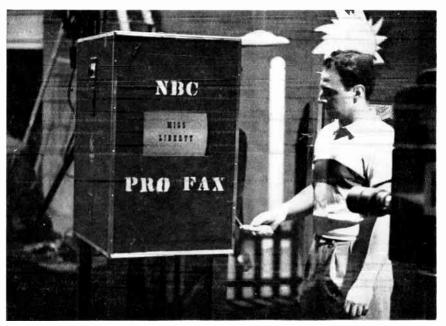
Fig. 9-12. NBC crawl-title device. Aperture in box,  $7\frac{1}{2}$  by 10 inches. Scanned area, 6 by 8 inches. NBC suggests using a safe title area of 5 by 6 inches.
