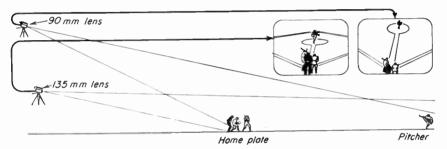
Fig. 20-31. Effect of camera height on cover shot.
