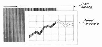
Fig. 13-10. One method of making a graph line slowly grow.
