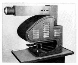
Fig. 10-9. Beseler OA4 opaque projector adapted for television. Optical system has been doubled back on itself to conserve space. This machine handles a picture size of 8 by 10 inches.
