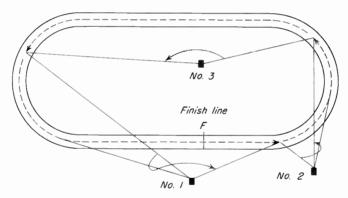
Fig. 20-25. WBKB race-track pickup with camera in the infield. Range of usefulness of each camera is shown.
