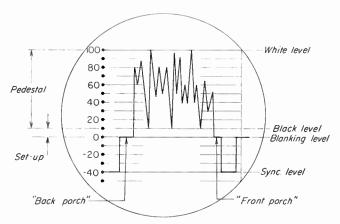
Fig. 15-14. Oscilloscope screen (also called waveform monitor, oscillograph, or C.R.O.).
