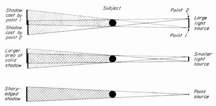
Fig. 12-21. Sharpness of shadow is determined by size of light source.
