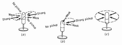
Fig. 19-4. 77DX used (a) as a bidirectional, (b) as a unidirectional, and (c) as a nondirectional microphone.
