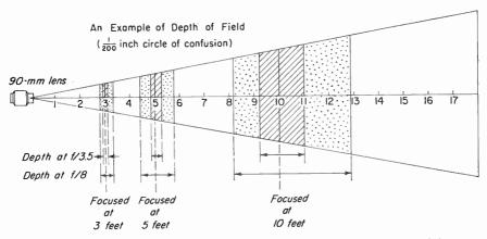
Fig. 5-26. Depth of field with the 90-mm lens. The farther the point of focus is from the camera, the greater the depth of field. Depth of field is increased by stopping down the lens.
