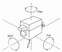
Fig. 4-3. Rotation around three camera axes.
