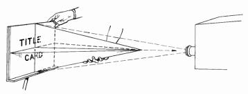
Fig. 9-4. Double T-square device to aid in lining up titles. Known as "Bretzaligner." Can be built of two pieces of cardboard, each notched halfway like dividers in an egg crate.
