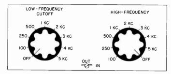
Fig. 19-22. Control panel of typical sound-effects filter.
