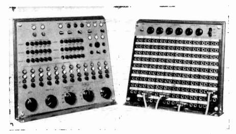
Fig. 19-26. Left panel and right panel (patchboard) of NBC television audio console.
