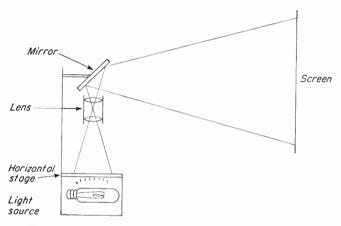
Fig. 13-5. Diagram of overhead transparency projector.
