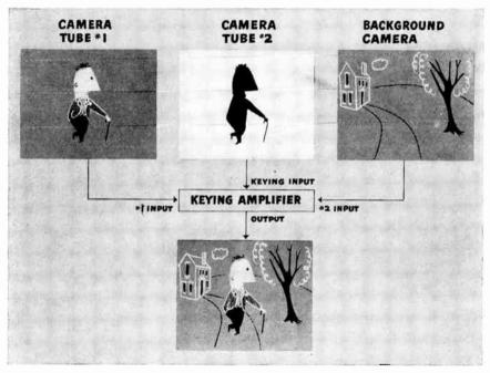
Fig. 15-12. VideoScene technique. The VideoScene camera is an adapted color camera in which two tubes are used. Tube 1 (left) photographs the actor against a special reflective background. The second tube produces a silhouette of the actor. This then becomes the keying signal which controls the electronic switching in the keying amplifier.
