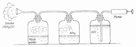
Fig. 14-5. Generator for ammonium chloride smoke.
