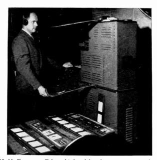
Fig. 10-11. Four-stage Telop; third and fourth stages are vertical at back.
