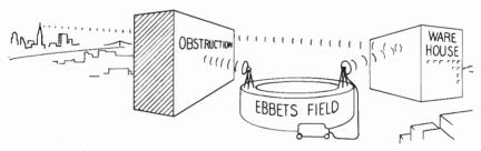
Fig. 20-8. Reflecting the beam is another method of getting the signal in when line of sight is lacking.
