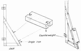
Fig. 16-4. Jack. This unit is hinged to the back of the flat and weighted at the bottom to keep the flat from falling forward. A sandbag may be used or a standard counterweight as shown.
