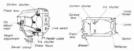
Fig. 18-10. Construction of Dyna-beam spotlight.
