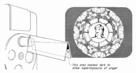
Fig. 11-22. Kaleidoscope used by NBC on "Garroway at Large."
