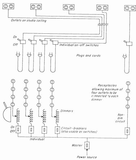
Fig. 18-15. Diagram of a simple patchboard. Only a few circuits are shown.
