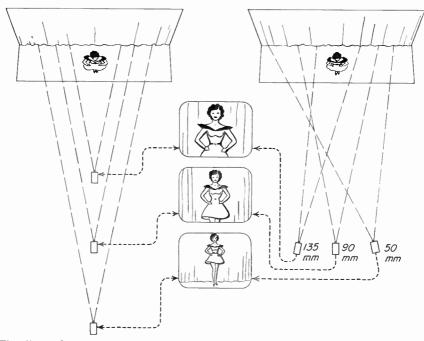
Fig. 5-1. Three standard shots—long shot, medium shot, and close-up—taken by (left) a 90-mm lens from three different distances and (right) three different lenses from the same distance.
