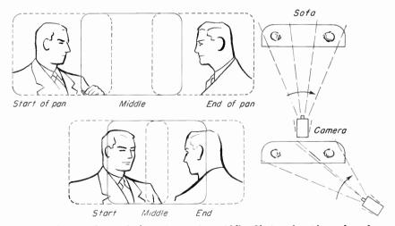
Fig. 4–4. The pan shot with the uninteresting middle. Choice of a side angle reduces the length of the pan. The new subject can start to enter the frame as soon as the camera starts to pan.
