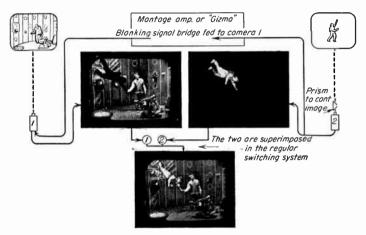
Fig. 15-7. Diagram of the Gizmo, first montage amplifier in regular broadcast use. Designed by Rolf Drucker, David R. Fee, and George Gould for use on "Tom Corbett, Space Cadet." Photos taken off control-room monitors.
