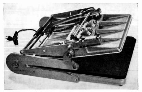
Fig. 9-25. Fotoflat dry-mounting press.
