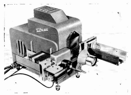
Fig. 12-16. The TelePro 6000 rear screen projector. This projector is equipped with an automatic remote-control slide changer, takes a maximum of sixty-five 3½- by 4-inch slides (including Polaroid transparencies), and changes slides in ½ second without black screen interval. Auxiliary slide holder (center, above projection aperture) allows single slides to be inserted manually at any time during slide sequence.
