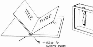
Fig. 9-7. Turning pages. Each page is attached to a stiff wire which is operated from the back.
