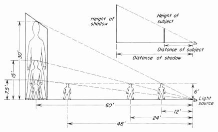
Fig. 12-20. Size of shadow varies inversely as distance of subject from light source.
