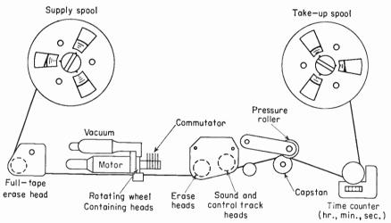
Fig. 23-3. The Ampex VTR 1001, a more compact and portable model than the VTR 1000, with a diagram of its tape transport mechanism. This is essentially the same as that of the first model.
