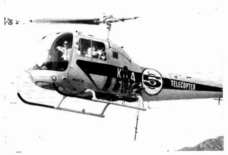
Fig. 20–20. KTLA Telecopter over Los Angeles. GE vidicon camera with Pan Cinor zoom lens and open frame view finder protrudes from cockpit window. Transmitter antenna, below, must be raised before landing.
