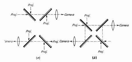
Fig. 10-6. The development of the more complex multiplexer. Two 3-input, 1-output multiplexers (a) facing in opposite directions are combined (b) to make a 4-input, 2-output multiplexer.
