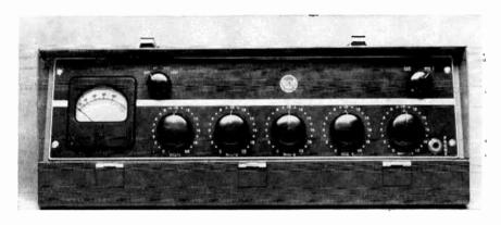
Fig. 20-9. RCA transistorized portable console BN6B. Four microphone positions and master gain are provided.
