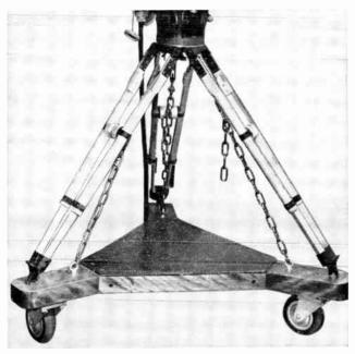
Fig. 4-8. Station-built tripod dolly with caster wheels. Lack of cable guards is serious disadvantage.
