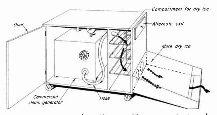
Fig. 14–8. Improved fog machine with commercial steam generator to produce greater quantities of steam and hence fog.
