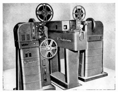
Fig. 1-3. A typical television film chain. Two 16-mm film projectors, optical system (multiplexer), and vidicon TV camera.
