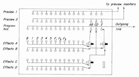
Fig. 7-6. Special five-bus switching system built by CBS.
