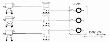
Fig. 7-1. Mixer type of switching system.
