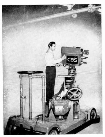
Fig. 4-16. Fearless dolly adapted by CBS with 3-foot extension on boom counterbalanced by large weight (foreground). Note that auto steering wheel replaces standard handle.
