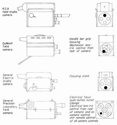
Fig. 3-1. A comparison of the major American makes of image-orthicon cameras. The GPL camera at the bottom is actually manufactured in England by Pye.
