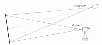
Fig. 12-17. Front projection from overhead with tilted screen.
