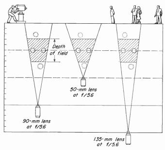
Fig. 5-30. Comparison between depth of field when same width of scene is maintained in shots taken by three standard lenses. You cannot improve depth of field by changing lenses unless you accept a wider angle of view.
