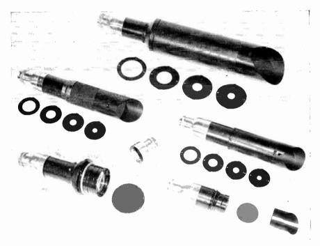
Fig. 5-2. A selection of field-camera lenses supplied by RCA. Lower right: 8½-inch lens with lens cap and sunshade; lower left: 13-inch f/3.5; center right: 15-inch; center left, 17-inch; top, 25-inch. Waterhouse stops (described on page 86) accompany the three largest lenses in stops of f/8, f/11, f/16, and f/22.
