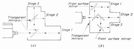
Fig. 13-2. Three-stage shadow box. (a) Two stages correct; one reversed. (b) Alternative design; no stages reversed.
