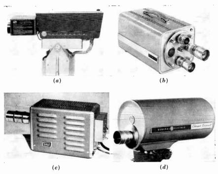
Fig. 3-6. A selection of four representative types of industrial vidicon cameras. (a) Hallamore, (b) Argus, (c) Dage 63A, (d) General Electric TE9A. Cameras b, c, and d are entirely self-contained, requiring no further equipment for operation. Camera in (a) is shown with remote-control pan and tilt apparatus and remote-control Zoomar lens.
