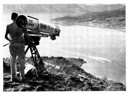
Fig. 5-7. A 110-inch lens at KOMO-TV, Seattle. Horizontal angle of view: 0.6 degrees. This is sufficient to fill the entire camera field with a close-up of the sun or moon. Here the lens is shown following hydroplane races on Lake Chelan.
