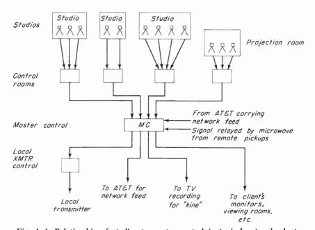
Fig. 1-4. Relationship of studios to master control in typical network plant.
