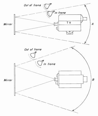
Fig. 9-5. Will lights glare off the title card? Imagine that the title is a mirror, and determine whether or not the lights would be in the mirror's field of view. (A) Vertical field of view, (B) horizontal field of view.
