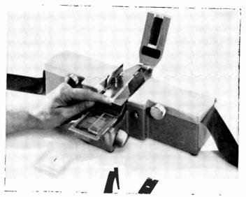
Fig. 23-6. A video-tape splicer made by Ampex. Pressure-sensitive tape is used to hold the two tape ends together, just as in audio-tape splicing.
