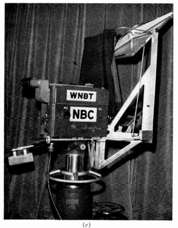
Fig. 11–4. Studio periscopes (a) for high-angle shot, (b) for low shot, (c) with adjustable top mirror attached to NBC camera.
