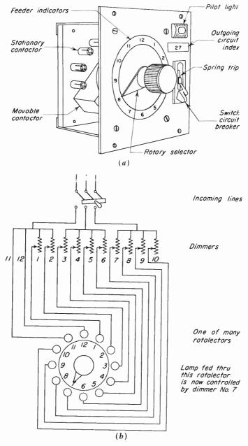
Fig. 18-17. The Rotolector unit and its relation to dimmer circuits. Each Rotolector is wired to the same dimmer circuits in this manner.
