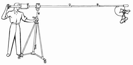
Fig. 19-16. Typical small giraffe boom.
