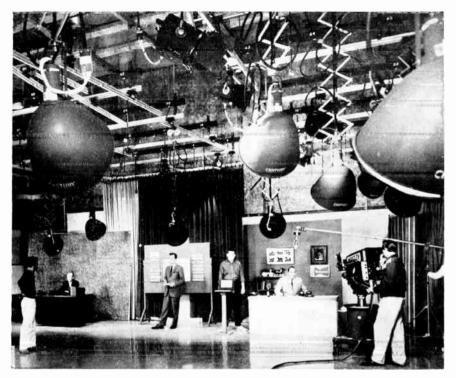
Fig. 18-12. Lights mounted on individual pantographs. Note use of short adjustable cross members on the grid. (Photo courtesy of NBC.)
