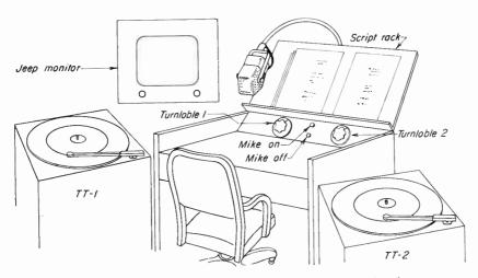
Fig. 19-21. Turntable equipment set up in announce booth.
