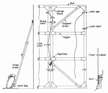
Fig. 16-2. The back of a plain flat, showing frame construction and standard hardware. Part of a second flat is shown at the left to indicate the method of lashing the two together.
