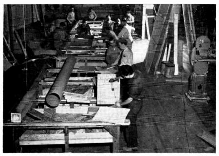
Fig. 16-18. Scene-construction shop, showing jig tables for flat construction. (Photo courtesy of CBS.)
