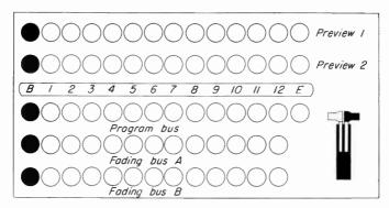
Fig. 7-5. Typical three-bus panel. Release off, or black, buttons at far left of each row are used for dissolving to black.
