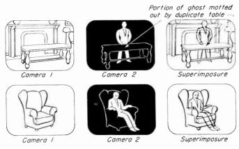
Fig. 15-2. Ghost effect complicated by necessity for ghost to move behind objects in the real scene. Solution is to have duplicate objects (black) in the ghost set.
