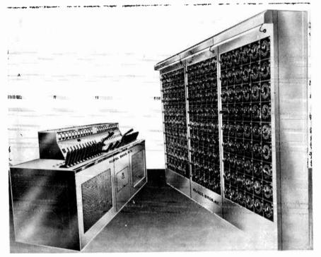
Fig. 18-18. Large Rotolector board at NBC, Hollywood. One hundred and seventy 24-contact Rotolectors are used: 24 dimmers.
