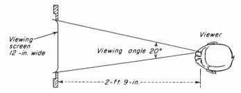
Fig. 5-18. Relationship of screen width and viewing distance to viewing angle.
