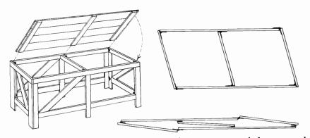
Fig. 16-9. Large platform, built of two parts for easy storage—platform top and parallel. Method of hinging parallel so that it will fold flat is indicated.
