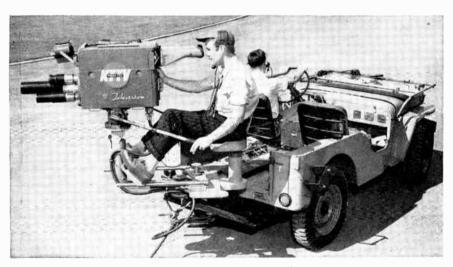
Fig. 20-28. KTTV camera mounted on jeep.
