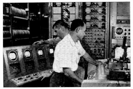
Fig. 23-7. The TV-Ola, left, operating in conjunction with a video-tape recorder, right. The four Tonotron tubes which freeze and hold the frames are seen at left; controls for selecting frame frequency are on the console at lower left.
