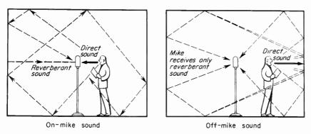
Fig. 19-2. When the ratio of direct sound to reverberant sound is high, the actor sounds "on-mike." When the reverberant sound becomes equal to or greater than the direct, however, the actor sounds "off-mike."
