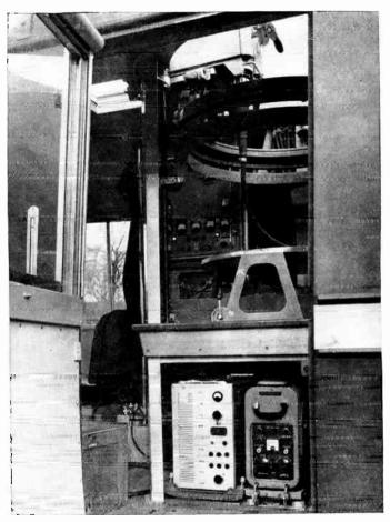
Fig. 20–17. Interior of BBC Roving Eye. Camera well and part of camera, which protrudes through roof, can be seen. Camera is roller-mounted on a circular track, so it may be swung around to face any direction, while the operator remains always behind it. Vertical adjustment screw shows at left of track.
