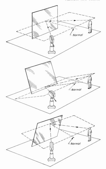
Fig. 11-13. The first law of reflection: The incident ray, the reflected ray, and the normal to the surface lie in the same plane.
