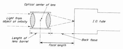
Fig. 5-22. Focal length is the distance from the optical center of the lens to the focal plane when the lens is focused on infinity. It is not to be confused with back focus or the length of the lens barrel.
