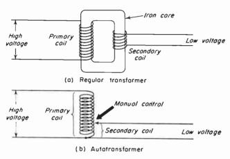
Fig. 18-14. Principle of autotransformer dimmer.
