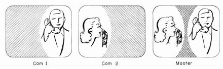
Fig. 12-9. Matting by off-setting the lens turret. The two cameras are superimposed for the composite effect shown at right as it is seen on the master monitor.
