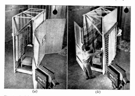
Fig. 16–13. (a) WTMJ-TV stage wagon carrying two sets. (b) stage wagon after being turned around, with another set open and ready to be used.
