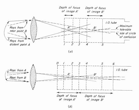
Fig. 5-28. Attempt to split focus between two objects is unsuccessful in (a) when lens is wide open, but succeeds in (b) when lens is stopped down. *Note:* Amount of movement of the tube is exaggerated for purposes of illustration. The possible length of travel is only a little over 2 inches.
