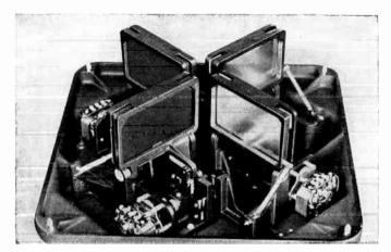
Fig. 10-5. Mechanism of the RCA TP15 multiplexer, an example of the four-input, two-output type. Mirrors hinge down for almost instantaneous change-over.
