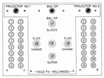
Fig. 10-1. Remote control panel with tally lights showing which slide is in place in each projector.
