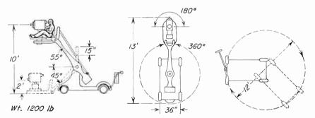
Fig. 4-20. Dimensions and range of movement of Houston crane.
