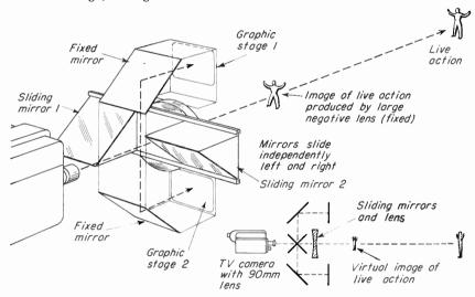
Fig. 13-3. Combination of shadow box and live action with mirror wipe. Designed by Karl Weger.
