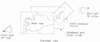
Fig. 13-15. Method of wiping in rear-lighted arrow.
