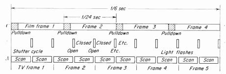
Fig. 10-12. The synchronization problems between film and TV. A typical method of fitting 24 film frames into 30 television frames. (The above chart shows four film frames and five TV frames, since ½ second is covered.)
