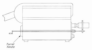
Fig. 11-15. Control for rotating prism from rear of camera.
