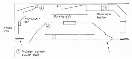
Fig. 16-1. Playing area at end of typical small television studio, showing four sets in place to demonstrate the process of *in-setting*. (1) Roll drop let down for background of show 1. (2) Set for show 2. (3) Permanent set for show 3. (4) Permanent set for show 4. (5) Traveler curtain may be pulled across for still another background.
