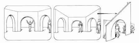
Fig. 12-5. The illusion of space obtained by building sets in forced perspective.
