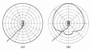
Fig. 19-8. Directional characteristics of the RCA 88A. (a) At 1,000 cycles it is nondirectional; (b) at 4,500 cycles it is almost unidirectional.
