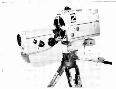
Fig. 5-13. Watson zoom lens (British make). Zoom ratio: 5 to 1, electrically controlled. Lens is first attached to tripod, then camera is placed on lens.
