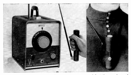
Fig. 19-15. Vega wireless microphone. Receiving unit on left. Mike may be used in the hand with telescoping antenna or may be worn as a lavaliere, in which case the neck strap acts as an antenna element. Several Vega microphones may be used with one receiving unit, either on the same frequency (in which case they all operate together without individual adjustment) or on different frequencies (in which case they can only be used separately, since the receiving unit must be retuned between them).
