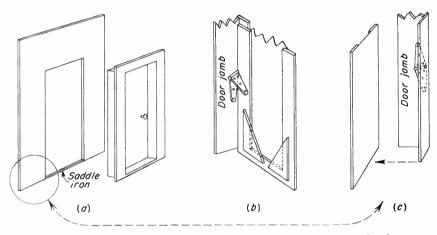
Fig. 16-5. Door flat and door plug, indicating method of securing the plug by means of a large strap hinge.
