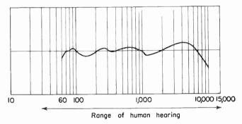
Fig. 19-9. Frequency response of the RCA 88A.
