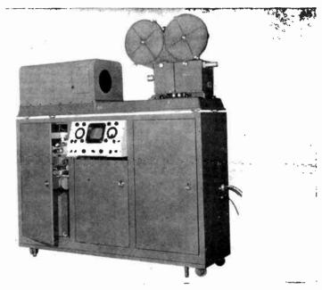
Fig. 23-1. Kinescope recorder made by GPL. A high-definition high-intensity monitor tube is enclosed in the housing at left. At right, focused on the monitor, is a specially built 16-mm motion-picture camera. Cabinet below houses sound equipment and chassis for the monitor tube.
