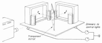
Fig. 13-1. Two-stage shadow box.
