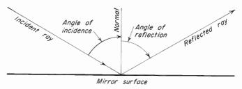
Fig. 11-11. The second law of reflection: Angle of incidence equals angle of reflection.
