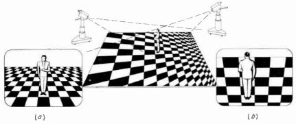
Fig. 12-4. Forced perspective seen from correct angle of view (a) and from the opposite angle (b).
