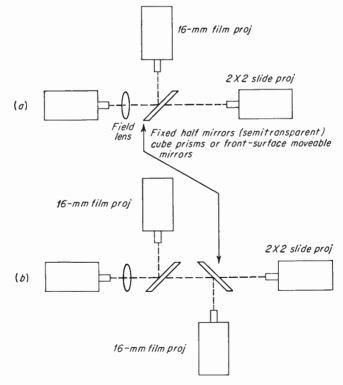
Fig. 10-3. Simple multiplexers. (a) A two-input, one-output multiplexer. (b) A three-input, one-output multiplexer.
