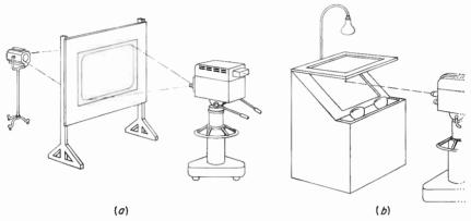
Fig. 13-16. Holden animator (a) as originally built with vertical stage, (b) with horizontal stage similar to Bretzicon.
