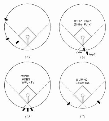
Fig. 20-32. Several methods of placing cameras, used experimentally in the first few years of televised baseball.
