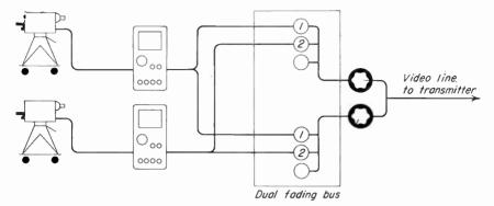
Fig. 7-2. Dual fading-bus type of switching system.
