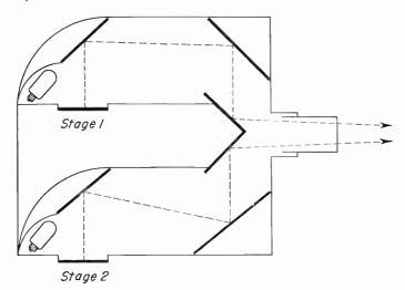
Fig. 10-10. CBS two-stage balop built from two standard Beseler OA2s.
