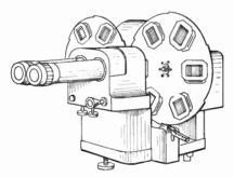
Fig. 10-7. Gray Telejector, a dual 2- by 2-inch slide projector holding 12 slides.
