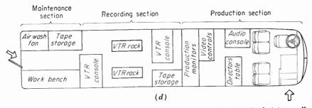
Fig. 20-18. Mobile video-tape van made by Crown Coach. (a) Technician pulls camera cable from reel on side of vehicle. (b) Rear view shows roof access. A video-tape console can be seen inside the vehicle. (c) Shelf for camera storage slides out for easy access. Camera and microphone inputs and video outlets are on panel at left. (d) Diagram of interior layout.
