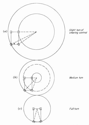
Fig. 4-25. Circular steering with the crab dolly. (a) With a slight turn of the steering control the dolly turns on a wide circle. (b) With a medium turn of the handle the circle is smaller. The center of rotation is still in line with the front axle. Note how the two steering wheels must turn different amounts. (c) With a full turn of the handle the dolly rotates around a point between the two front wheels.
