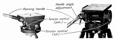
Fig. 4-5. Two of the best friction heads: Fearless (left) and Camera Equipment Co. (right).
