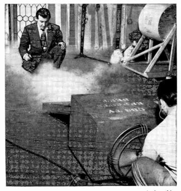
Fig. 14-7. Simple fog machine. Boiling water creates steam which is blown across dry ice to condense into fog.
