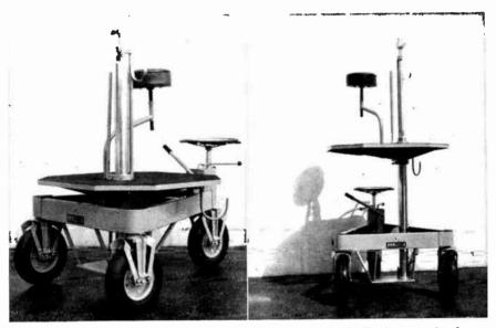
Fig. 19-18. Fisher microphone boom base. Designed specifically for TV, this boom perambulator features a circular platform (operator can't fall off from panning the boom too far); cable guards, shown in raised position (operator can't fall off because of sudden stops against cables); and 3-wheel synchronous steering (maximum maneuverability). It is also provided with a braking mechanism.
