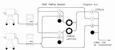
Fig. 7-3. Three-bus type of switching system.
