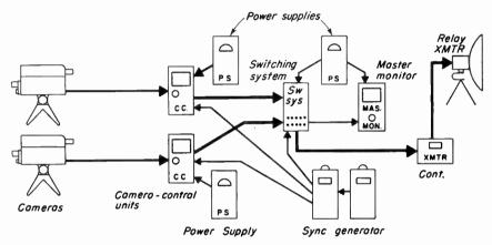
Fig. 20-3. Diagram of video equipment for two-camera remote pickup. (RCA equipment shown.)
