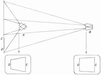
Fig. 9-2. (A) Camera in near position with wide-angle lens. Effect of keystoning is noticeable (square or rectangular area takes a keystone shape). (B) Camera in more distant position with long lens. There is less keystoning because camera covers the sides of the picture from more nearly a perpendicular angle.
