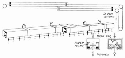
Fig. 16-8. Travelers for traveler curtains. Either rollers or balls may run in the track. One cord moves both curtains.
