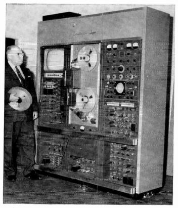
Fig. 23-4. The RCA video tape recorder is similar to the Ampex except that it is rack-mounted.
