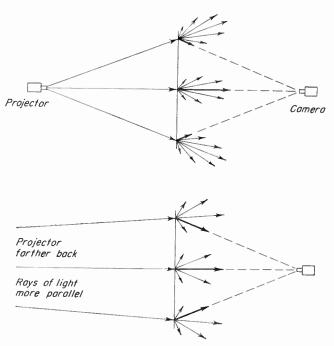
Fig. 12-14. Diffusion pattern from three rays of light, one central and one at each side of the screen. When the projector is close to the screen, the sides of the picture are dark; when the projector is farther back, the screen is more evenly illuminated.
