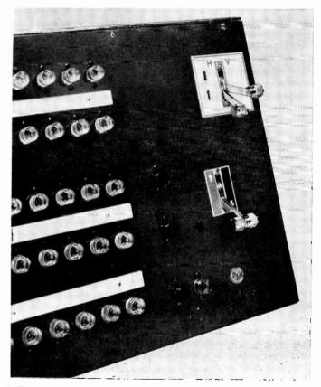
Fig. 15-5. Wipe control handles on a five-bus switching system. Top: Wipe selector busses with horizontal and vertical wipe control handles. Middle: Two effects busses with dissolve handles. Bottom: Program bus.
