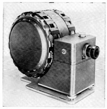
Fig. 10-8. RCA TP7 slide projector, a dual 2- by 2-inch slide projector utilizing one light source and one projection lens. Magazines hold total of 36 slides.
