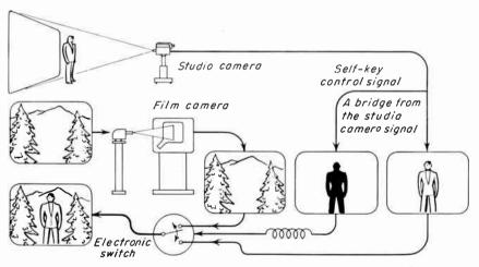
Fig. 15-8. Simplified diagram of a second type of montage amplifier.
