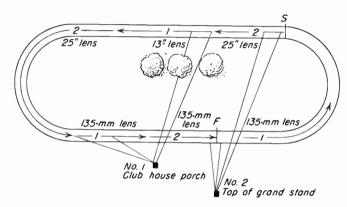
Fig. 20-26. Camera placements for WDSU-TV two-camera pickup at New Orleans track.
