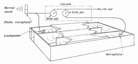
Fig. 19-23. Typical echo chamber.
