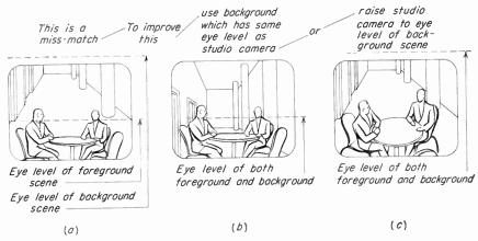
Fig. 12-12. Perspective in rear-projected background scenes must match the foreground. In (a) the two do not match; (b) and (c) indicate two solutions to the problem.
