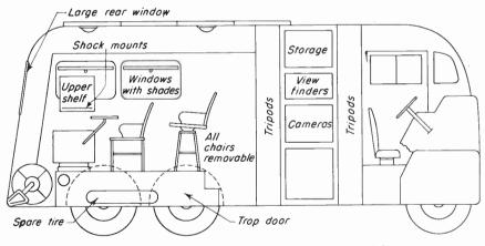
Fig. 20-14. Plan and elevation of General Electric mobile unit.
