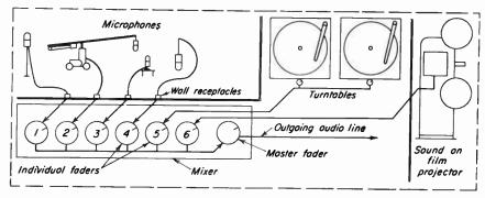
Fig. 19-1. Diagram of audio equipment in the typical small television studio.
