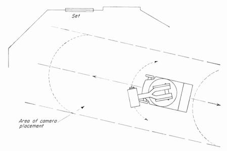
Fig. 4-14. A more flexible method of using the Panoram dolly. Camera has great freedom of positioning, and cameraman has freedom of forward and backward movement.
