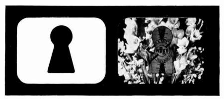
Fig. 15-9. Keyhole area used as control signal to make composite of two pictures.
