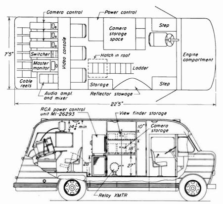
Fig. 20-12. Plan and elevation of RCA mobile-unit truck.
