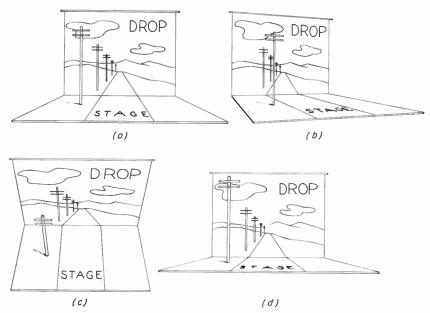
Fig. 12-2. Painted perspective in the drop will match the actual three-dimensional construction on the stage only if seen from the correct point of view (a). In (b) the illusion is lost because the viewpoint is too far to the side; in (c) too high; in (d) too low.
