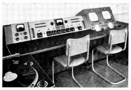
Fig. 19-19. RCA Consolette. Typical small console.
