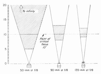
Fig. 5-29. Comparison between depth of field in three standard lenses focused on a point 10 feet distant.
