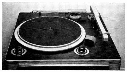
Fig. 19-20. Typical control-room turntable. Two pickup arms are included. The one at the back is a special lightweight arm for long-playing microgroove records. Left knob, speed selector; right knob, lateral or vertical cut selector.
