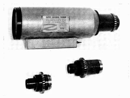
Fig. 5-12. Super Universal Zoomar with converters. Focal length of lens as shown above:  $2\frac{1}{2}$  to 16 inches (f/3.9). With converter at lower left: 4 to 25 inches (f/5.6). With converter at lower right:  $6\frac{1}{2}$  to 40 inches (f/8).
