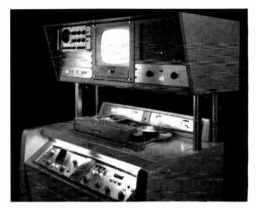
Fig. 23-2. The Ampex VTR 1000 video-tape machine.
