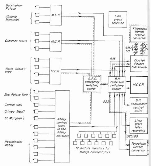
Fig. 20-34. Simplified schematic of BBC arrangements for
