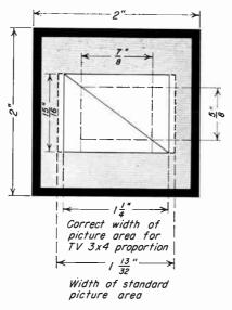
Fig. 9-28. Standard 2- by 2-inch slide with framing dimensions. Picture area for TV means scanned area. The safe title area is figured here on the basis of a  $\frac{1}{6}$  loss at each border rather than  $\frac{1}{10}$ , making is somewhat safer (see p. 138).
