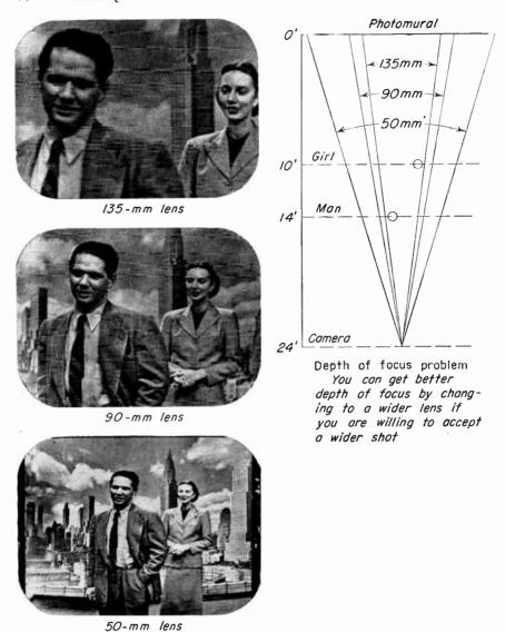
Fig. 5-14. Three shots taken from one camera position with three different lenses. Note that relative size of man, girl, and building remains the same. Only the field of view changes. Note also the improved depth of field in the wide-angle shot. (All lenses were opened to f/3.8 to exaggerate this difference in depth of field.)
