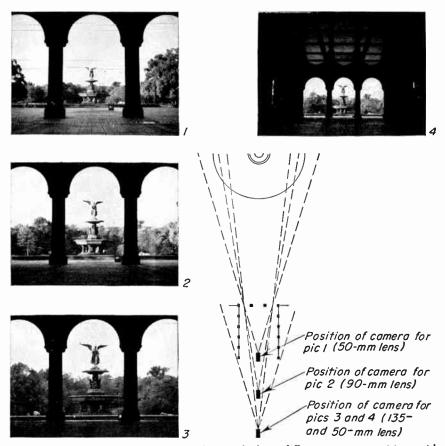
Fig. 5-16. Three shots, Nos. 1, 2, and 3, made from different camera positions with different lenses, keeping the arches the same size. Note that wide-angle shot 4 from same camera position as 3 shows the same relative size of fountain and arch.
