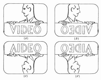
Fig. 15-13. Three types of scanning reversal. (a) Straight shot; (b) horizontal reversal; (c) vertical reversal; (d) horizontal and vertical reversal.
