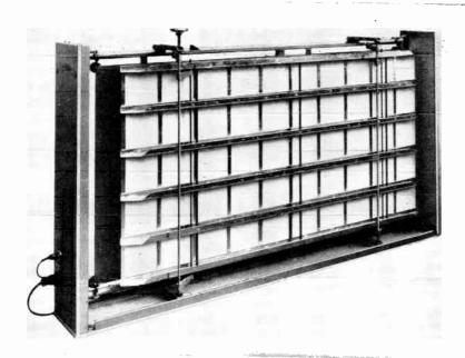
Fig. 19-24. Artificial reverberation apparatus, made by E.M.T., West Germany, shown with cover removed. A flexible metal plate (black) is suspended behind white porous damping plate. Handwheel at top sets amount of damping and thus controls echo time.
