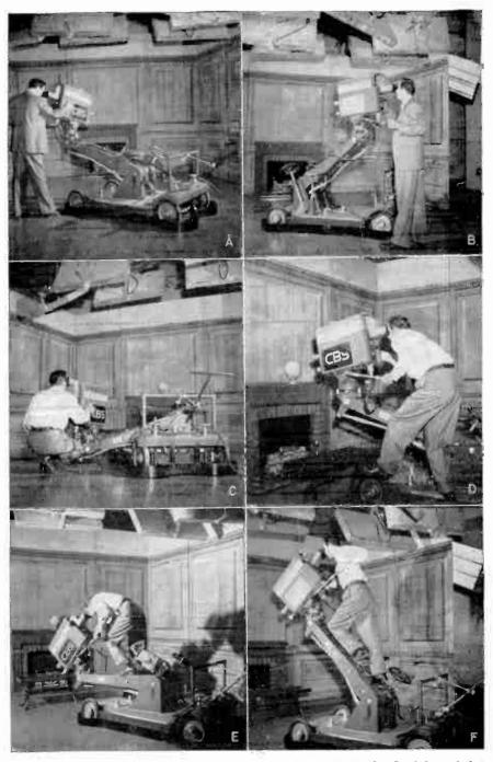
Fig. 4-15. Howard Hayes, top CBS cameraman, demonstrates the flexibility of the camera when mounted on the Panoram dolly.
