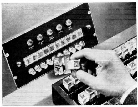
Fig. 15-6. A wipe effect with printed circuit attached is selected from RCA kit of 150 types. After removal of selector panel face plate, it may be plugged in to replace one of the 10 now in position.
