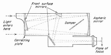
Fig. 5-6. Sketch of interior of Video Reflectar lens. Exposure control is accomplished by means of a simple damper. When this is horizontal, the lens is rated at f/8.
