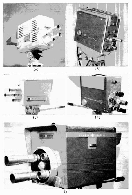
Fig. 3-7. Several representative examples of studio vidicon cameras intended for broadcast purposes. (a) Dage 320A, (b) RCA TK15, (c) Kintel, (d) GPL PD250, (e) General Electric TG2.
