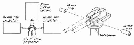
Fig. 10-2. Multiplexer for use with iconoscope film-pickup camera. Four projections are imaged on camera tube, each one slightly off camera axis, causing unnoticeable keystoning.
