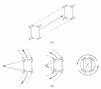
Fig. 4-22. The two steering modes of the Sanner dolly. (a) Synchronous steering. (b) Differential steering.
