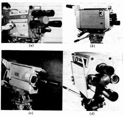
Fig. 3-8. Four major makes of 4½-inch image-orthicon cameras. (a) E.M.I. (Electro-motive Industries, British), (b) Pye (British), (c) Marconi (British), (d) RCA.
