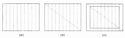
Fig. 9-14. Sherwin method of determining copy (essential) area. (a) Total scanned area (dead-border area may surround this). Scanned area is divided into 10 vertical segments. (b) Diagonal is drawn from corner to corner to locate corners of the safe title area. (c) Top and bottom of safe title area are drawn.
