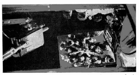
Fig. 11-5. Above, top-shot periscope in use on CBS show. Below, mirror on floor in NBC's "Cameo Theatre" reflects top shot from mirror on ceiling.
