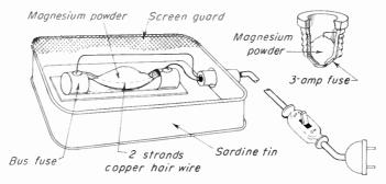
Fig. 14-15. Two ways to prepare magnesium-powder flash pots.
