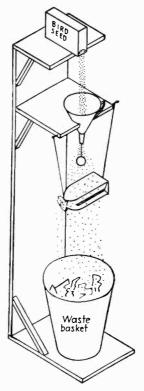
Fig. 49. A variety of the rain machine. A rapidly revolving disc may be used to distribute the birdseed, replacing the funnel, ping-pong ball, and paper bag used above.
