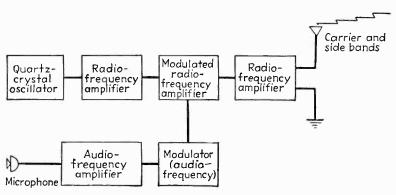
Fig. 15. Radio transmitter.
