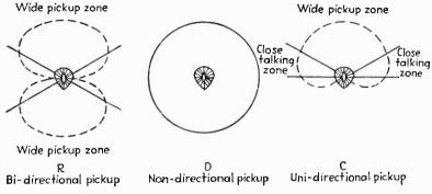
Fig. 7. Cardioid directional microphone.
