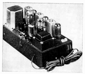
Fig. 56. Wired radio transmitter, 5 watt. (University of Michigan.)
