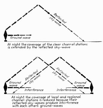
Fig. 16. Reflected sky wave—ground wave.
