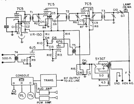
Fig. 58. Wired radio transmitter-schematic.
