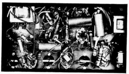
Fig. 57. Wired radio transmitter, 5 watt-bottom view. (University of Michigan.)
