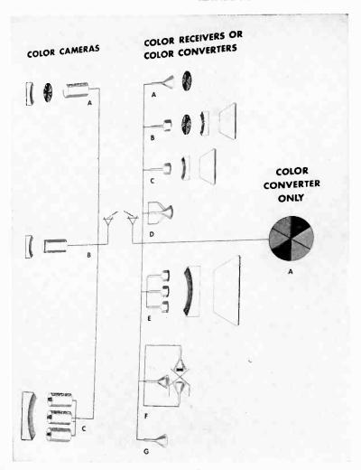
Fig. 25b. Chart illustrating the universal flexibility of the C.B.S. color television system. In the left column, A represents the present C.B.S. single-tube camera and lens with color disc; B is a C.T.I. type of camera, and C the R.C.A. 3-tube camera. All can be used in the C.B.S. color system; the C.T.I. and R.C.A. cameras, when and if they are perfected and made economically feasible.
