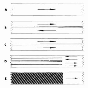
Full track. Mono recording is made across the whole width of the tape. Tape cannot be turned over
