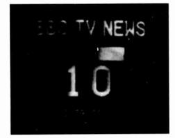
Figure 88 The countdown clock is displayed on screen before the start of the report. The white block moves from left to right to show the tape is running. The figure in the centre counts down the seconds and the time code at the bottom counts up the hours, minutes, seconds and frames. When the time code reaches zero (24) the report will go on air (courtesy BBC)
