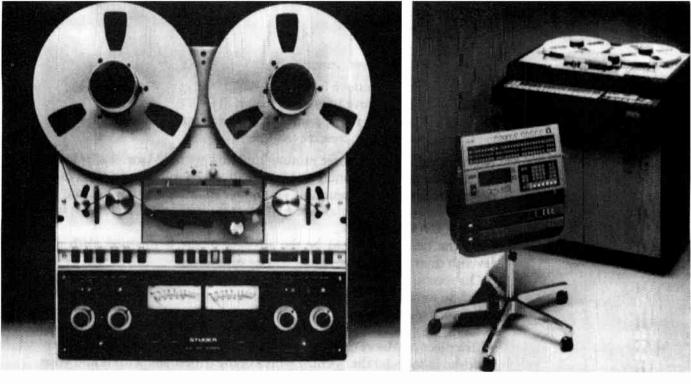
**Figure 53** (*left*) The Studer tape deck is the standard workhorse in many British radio stations. It features a counter for timing tapes and a built-in editing block for manual cutting and splicing. This machine is stereo (courtesy FWO Bauch Ltd, Studer Agents) (*right*) Digital technology is fast taking over in the studio, offering superior reproduction, computerized tape-handling and a sound quality that will not deteriorate over generations of recording (courtesy of Sony Broadcast Ltd)
