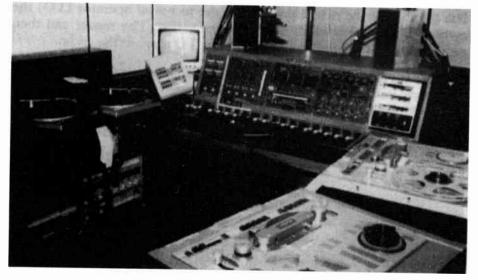
**Figure 57** (*above*) BBC Mark 3 control desk with grams and tape decks at BBC Radio Bedfordshire. (*right*) The on-air studio at Chiltern Radio, a British station in the independent radio network. The control desk is simpler and less cluttered than that used by the BBC. Commercials are kept on scores of cartridges – six are lined up in the machine (left) ready to go (Andrew Boyd)
