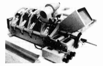
Figure 90 The Steenbeck flatbed editing machine permits the editor to review the film on screen while listening to the soundtrack (Andrew Boyd)
