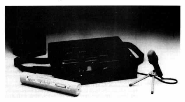
It is important *not* to stretch the cable so tightly that you tug at the connection into the tape recorder or the point where the cable enters the mike. These two electrical connections form the weakest part of the cable. It is easy to cause an electrical click on the recording or damage the connection by pulling at the lead.
