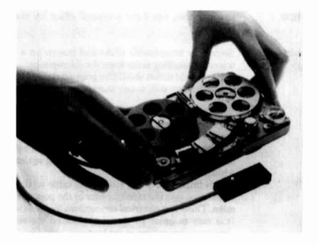
Figure 50 Nagra SNN miniature tape recorder – reel-to-reel quality at cassette recorder size (courtesy Kudelski)
