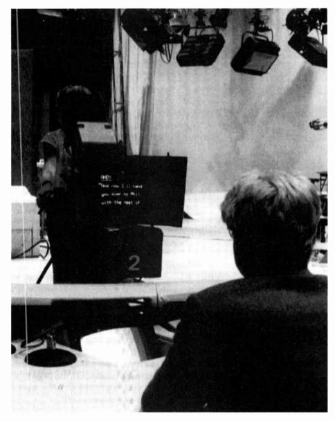
Figure 27 The studio teleprompter. The aim is to give the impression of eye contact with the viewer (courtesy EDS Portaprompt)
