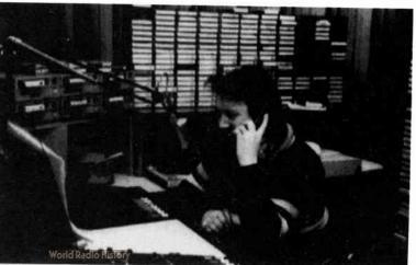
Standard equipment includes a control desk; two or more record decks, tape decks and CD players; several cart playback machines; cassette machine; monitor loudspeakers; telephone; talkback system, which is a form of intercom; presenter mike and possibly other microphones; studio clock with on-air lights, and in commercial stations, cart racks for adverts.
