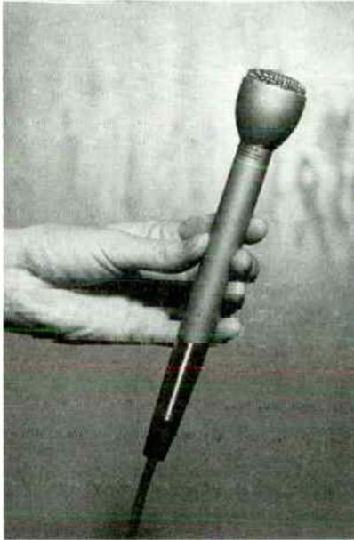
Figure 4.5 The RCA 77DX, a fine-quality ribbon mic.
