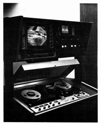
FIGURE 1.82 A videotape recorder
