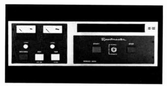
FIGURE 2.24 An audio cartridge record-playback machine
