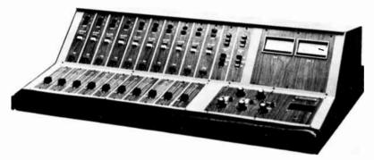
FIGURE 2.16 A mono radio board
