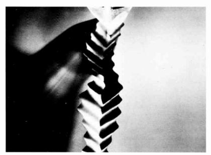
FIGURE 2.22 A magnified view of a quad disc groove. The small waves give third and fourth channel information; the major sidewall movements give stereo information.
