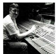
Producer/engineer Frank Filipetti is shown mixing the audio portion of James Taylor's "Live At The Beacon Theatre" DVD Video release at Right Track Studios in New York on a Neve Capricorn digital console. Not shown is the Sony 3348-HR multitrack recorder, which—like the Capricorn—operates at 24-bit resolution.
