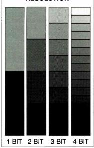
Figure 1. As the above graph illustrates, one-bit increments result in a doubling of the level of resolution. Accordingly, a 24-bit system, à la DVD Audio, offers 256 times the audio resolution of the CD, which has a word length of 16 bits.
