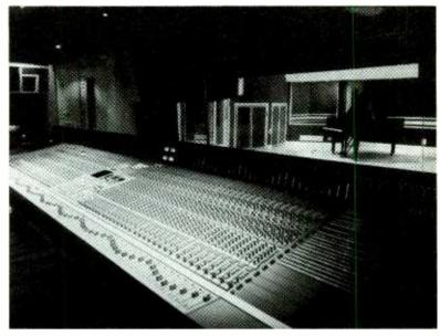
Abbey Road Refurbished. Abbey Road's Studio 3, above, was recently refurbished to include the first 72-input Solid State Logic SL8000 G Series multiformat production console in the U.K. The new board also features SSL's Ultimation console automation system.
