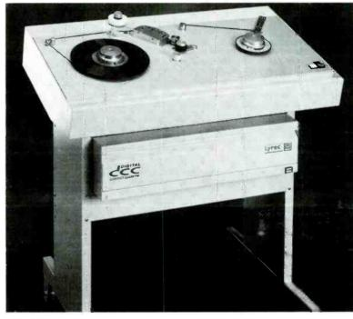
Above, Lyrec slave for high-speed DCC duplication has a suggested price of \$35,000 and is slated for May availability. The initial duplication ratio for DCC will be 64:1, while Otari, right, introduced the AL-632 loader, which can be converted to DCC duplication. Also introduced was the AL-662 double-pancake DCC loader designed primarily for manufacturers of blank tane.
