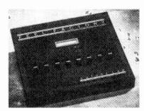
The new Feel Factory is the latest device to try to put more humanity into electronic music tracks. Its eight sliders are assigned to independent MIDI channels or notes, allowing the user to manipulate MIDI information in real time using proprietary algorithms.
