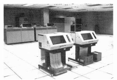
The nerve center of Camelot Music's new management information systems complex houses all of the department's equipment. Printers in the foreground generate bar code and pricing labels that are placed on product before shipment to stores. In the background are the company's two IBM System 38 computers.
