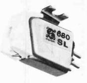
STANTON CARTRIDGE—Stanton Magnetics of Plainview, N.Y., has developed the model 680SL cartridge for use either in discotheques or in audiophile home stereo systems. The unit featues a patented "Stereohedron" stylus tip said to insure longer life to record collections. Weighing 5.5 grams, the unit has a tracking force of between two and five grams, and a frequency response of from 20Hz to 20kHz.
