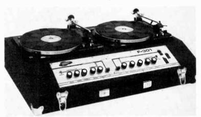
DISCO CONSOLE—This Farralane disco console features low noise integrated circuits, has harmonic distortion of less than 0.3% and a frequency response of 50Hz to 38kHz minus 3dB. The unit utilizes BSR model C206 belt driven turntables with strobe and pitch controls, viscous damped cueing, speed and anti-skate controls. It sells for \$775.
