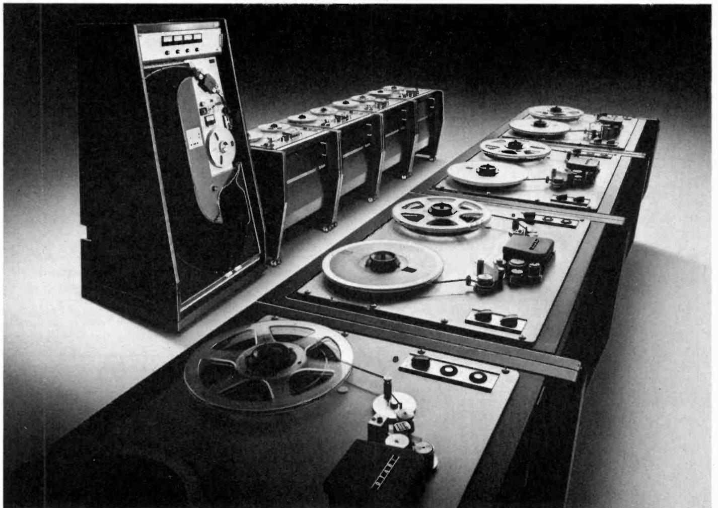
OTARI's DP-6000 duplicator is designed for quality sound duplications at the super high speed of 64:1! Its uniquely slanted loop bin insures smoothest 240 ips transport of your 3 3/4 ips master. Up to 10 slave units are centrally and automatically controlled. A quartz-crystal bias generator is employed, and crystal-coated ferrite heads assure clean, clear duplications for years on end. The high-performance system is also available at the 32:1 duplicating speed.
