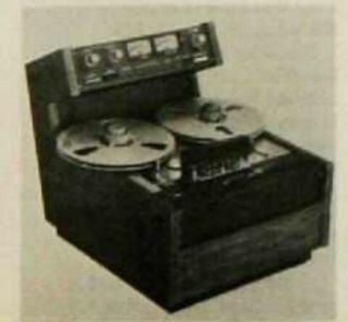
Otari Mark II professional recorder, a new generation of compact decks, offers 14-inch 2-channel or 1/2-inch 4-channel model, both with built-in DC servo, pitch control, separate transport and electronics, interface jack for dbx or Dolby noise reduction
