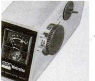
BSR introduces its Music Sound Level Meter which has a built-in microphone, calibrated VU meter and sensitivity control matching the meter to sound levels of up to 110dB. A test record is also included.
