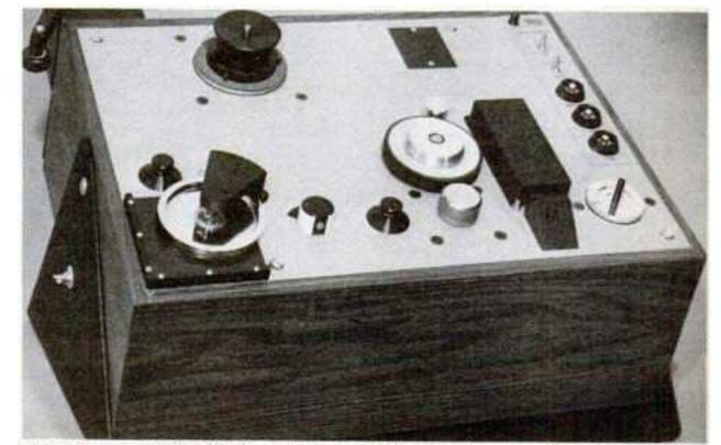
ED-PIC's new W25 300 ips winder includes a unique constant tension that measures largeness of supply reel and feeds information to the holdback tension and braking circuitry. Other features are flying anvil type cutter and a larger pinch roller.
