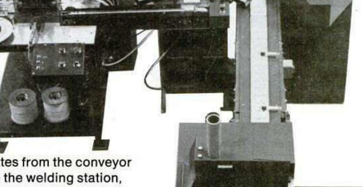
The In-Line Welder takes the cassettes from the conveyor belt and automatically advances them to the welding station, where they are sonically welded and ejected onto the packing surface. It's here where a final Quality Control check is made.
