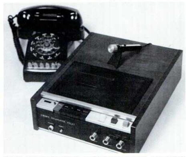
CROWN TELEPHONE VALET, imported and marketed by Industrial Suppliers, answers the phone and receives messages. Model 4400 accepts calls with a pre-recorded 20-second message. The caller's message is then recorded on a voice-activated cassette. After 8 to 15 seconds of silence, the machine is automatically shut off, ready for the next call. The 20-second message is pre-recorded on a continuous loop cartridge. The cassette recorder also doubles as a home player/recorder.
