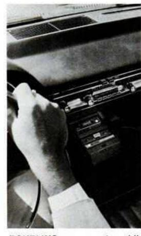
DOUBLING as an automobile entertainment system, the Carry-Corder can be used with Norelco's car mount, CMU 160. The unit plays through the car radio via the automobile electrical system and antenna connector. The Carry-Corder at any time can be easily removed from the stationary mount for portable use through its own batteries.
