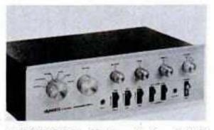
FLEXIBILITY is the forte of this new solid-state preamplifier, says builder Dynaco, Inc. It has headphone output, front panel input for electric guitar with mixing between channels and provision for simplified tape monitoring. And there is a "special" input permitting adjustment for a wide variety of additional functions. It's model PAT-4. Dynaco Inc., 3912 Powelton Avenue, Philadelphia, Pa. 19104.
