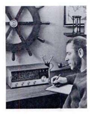
ZENITH'S EXPLORER, priced to sell at \$99.95, has five-band AM-LW-SW tuning with illuminated dial scales, bandspread dial and control, sensitivity switch, receive-standby switch, BFO on-off, automatic noise limiter on-off controls, line voltage selector switch, tuner output and headphone jacks and two antennas.
