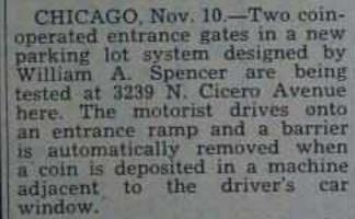
With insertion of the coin, the ramp moves four feet to one side, allowing the car to by-pass the barrier. The same type ramp is provided for the exit. When the lot is filled, a counter previously set for lot capacity shuts off the coin mechanism. Deposits in the exit ramp subtract from the entrance counter, allowing an equal number of cars to enter as others
