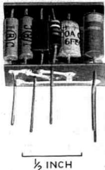
Fig. 47 — Small component module.
