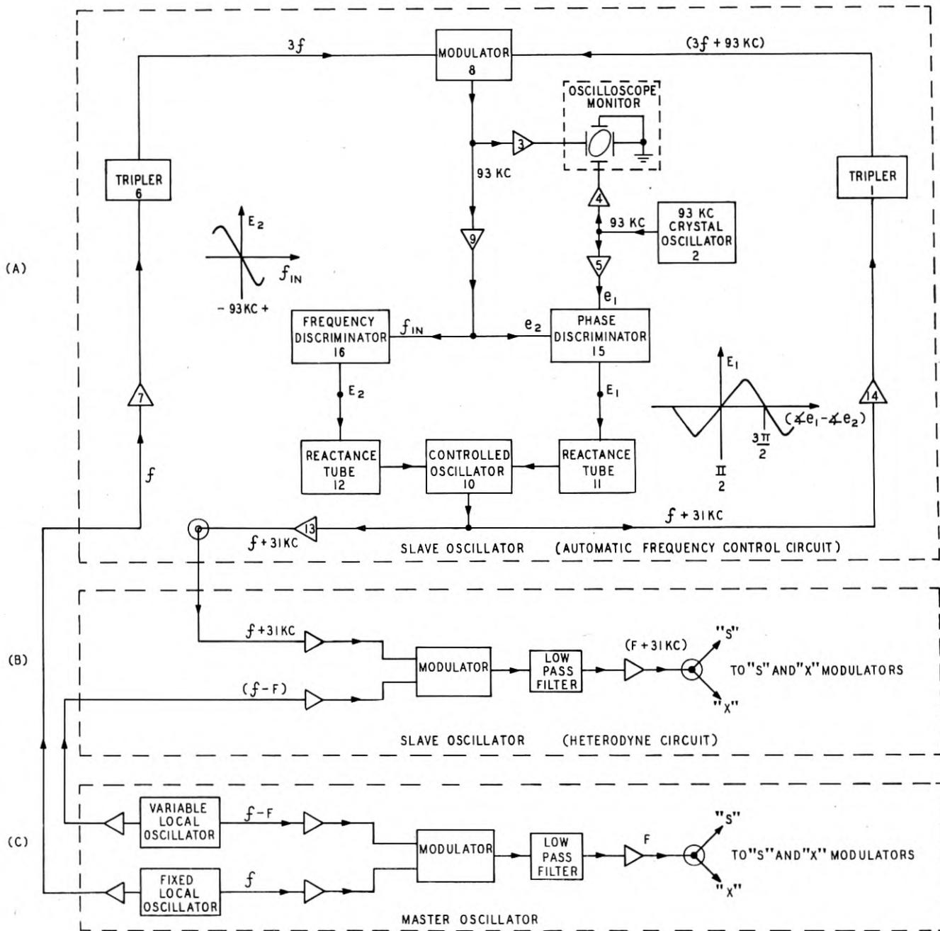
Fig. 5—Master and slave oscillators.
