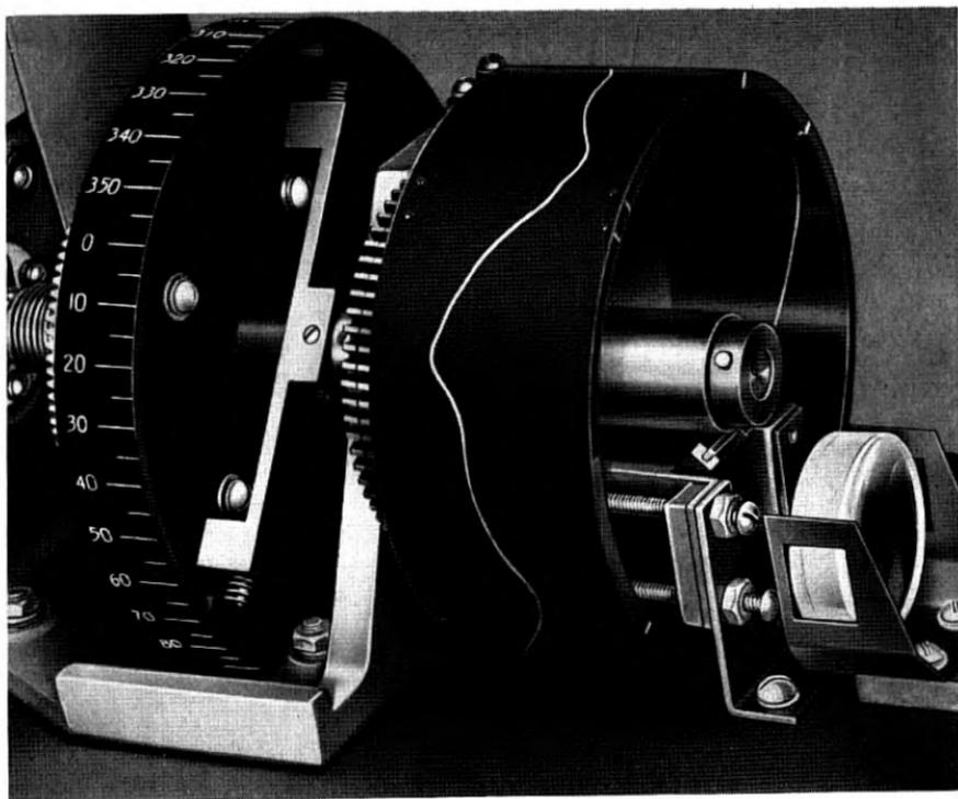
Fig. 10—Optical cam of phase shifter.
