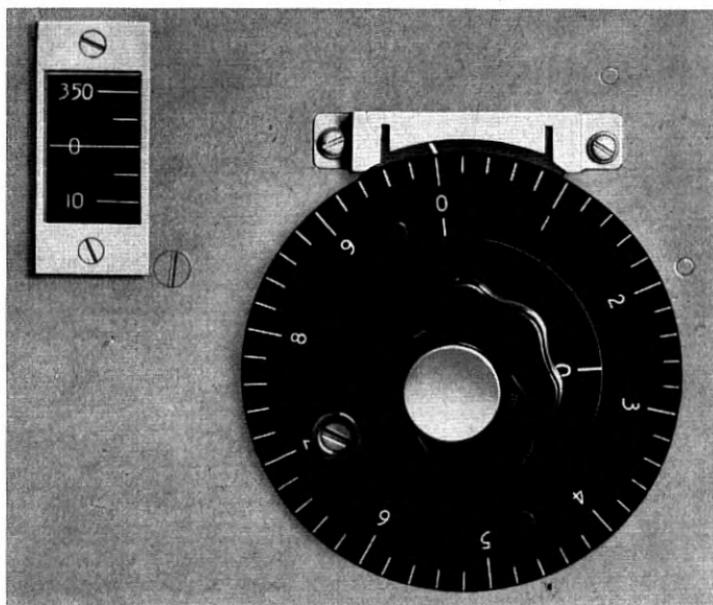
Fig. 11—Phase shifter scales and projected index.
