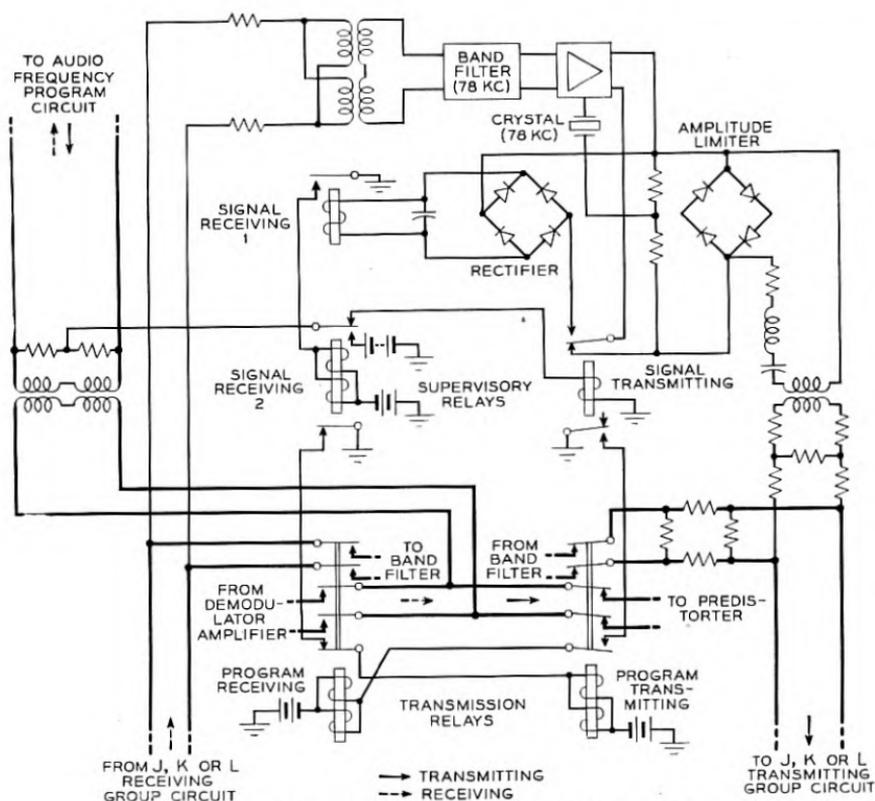
Fig. 4—Schematic of reversing and control circuit.
