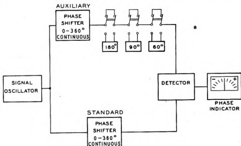
Fig. 12—Phase shifter calibration circuit.
