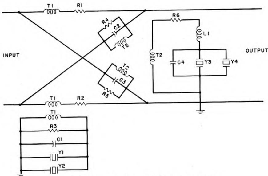
Fig. 14—Schematic of carrier-frequency equalizer.
