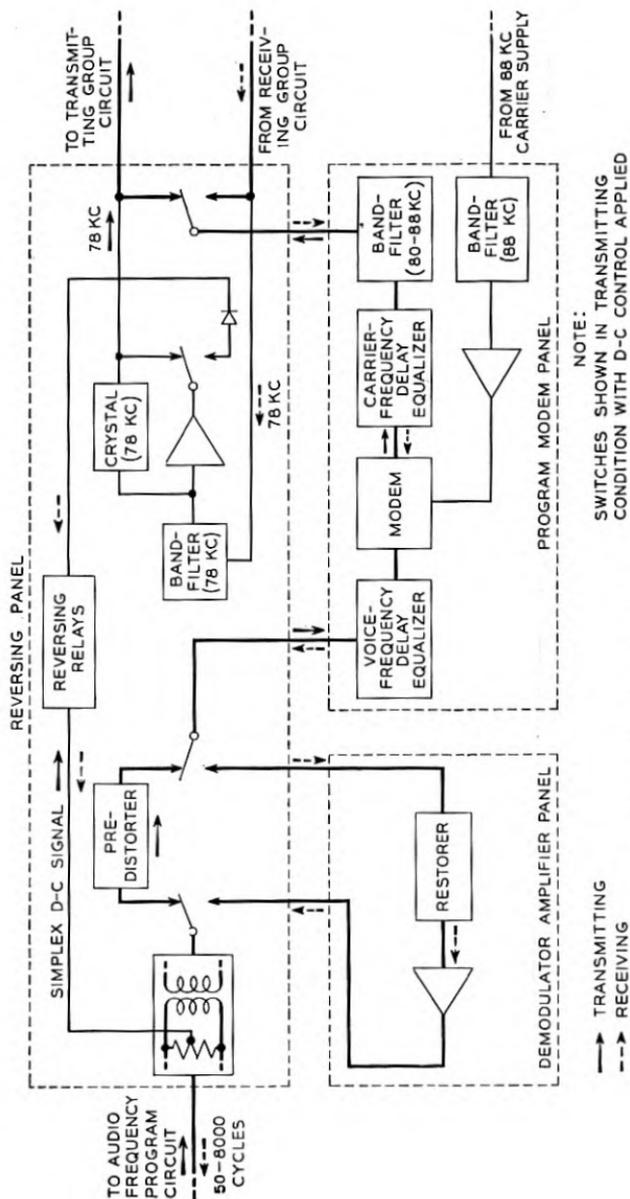
Fig. 2—Block schematic of carrier program terminal.
