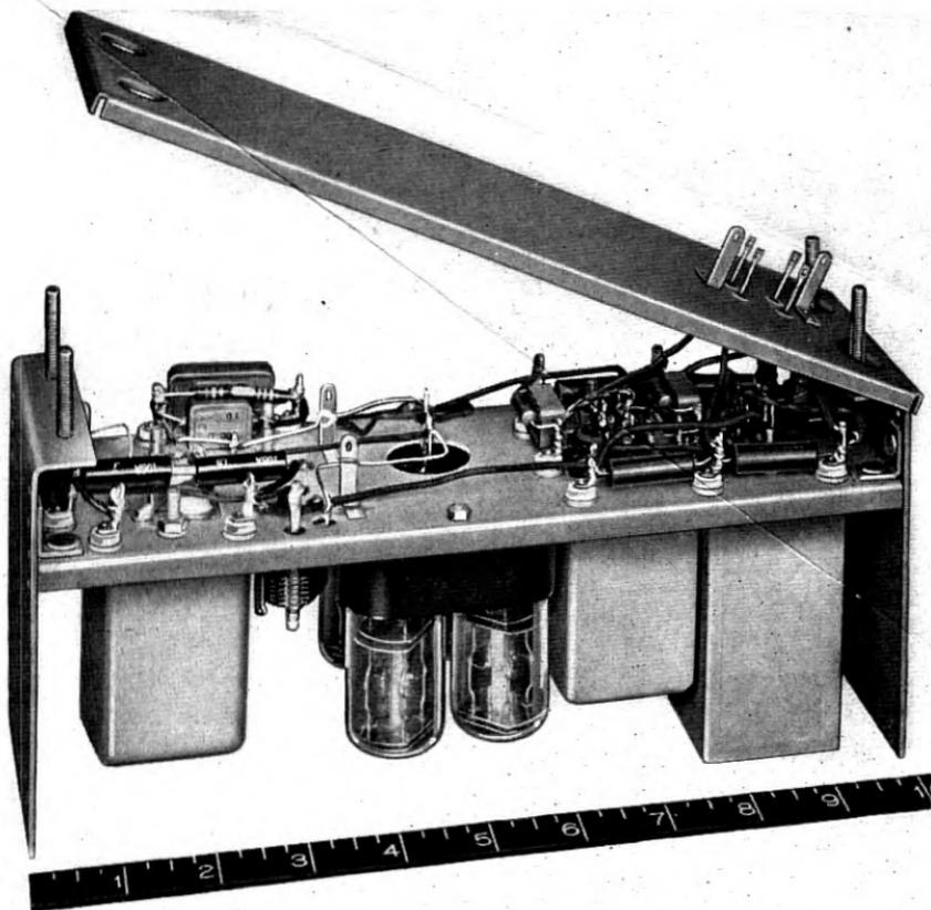
Fig. 15—Photograph of carrier-frequency equalizer.
