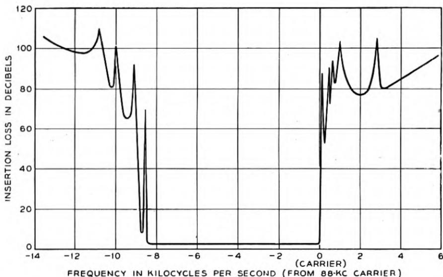
Fig. 2—The insertion loss-frequency characteristic of the filter.
