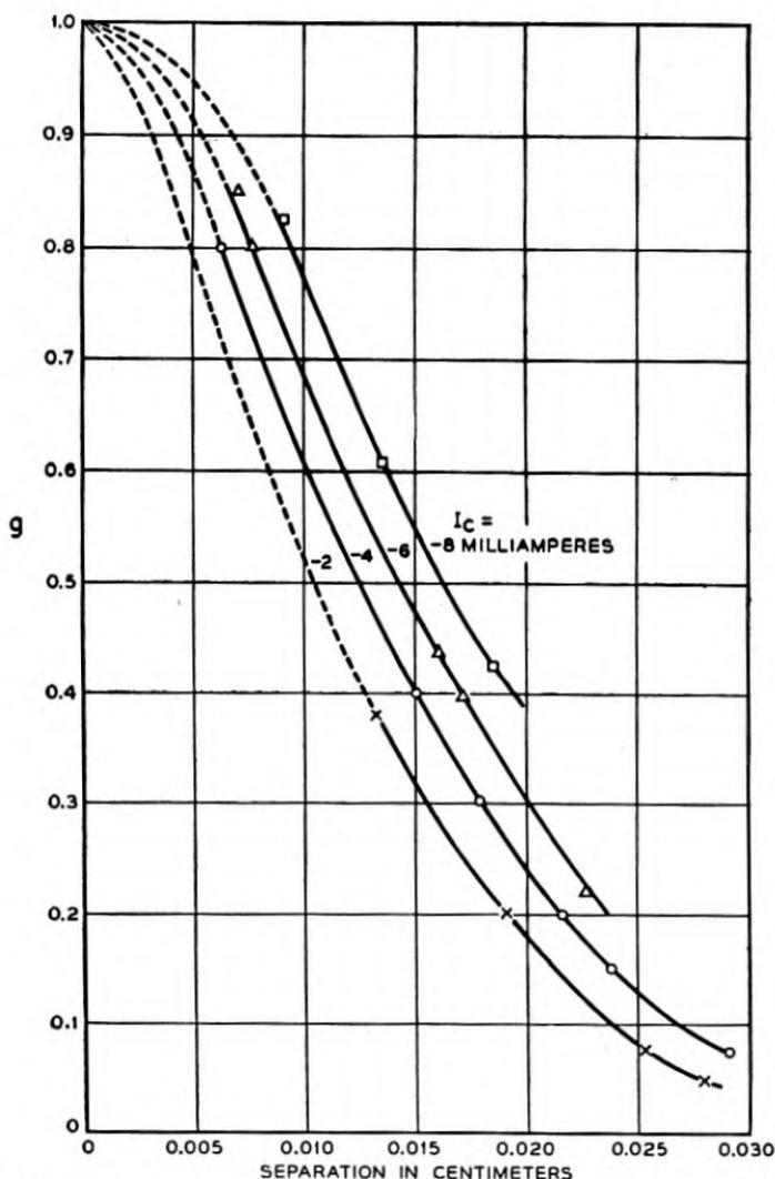
Fig. 9—The factor  $g$  is the ratio of the emitter current extrapolated to  $s = 0$  to that at electrode separation  $s$  required to give the same collector current,  $I_c$  and voltage,  $V_c$ . Plot shows variation of  $g$  with  $s$  for different  $I_c$ . The factor is independent of  $V_c$  over the range plotted.
