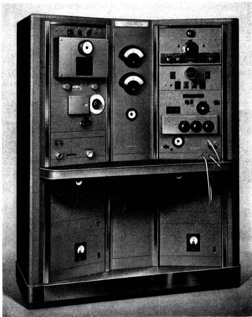
Fig. 4—The assembled phase and transmission measuring system.
