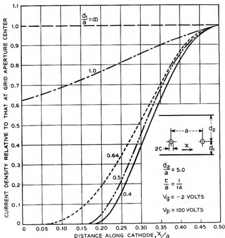
Fig. 4—Variation of current density in a triode.
