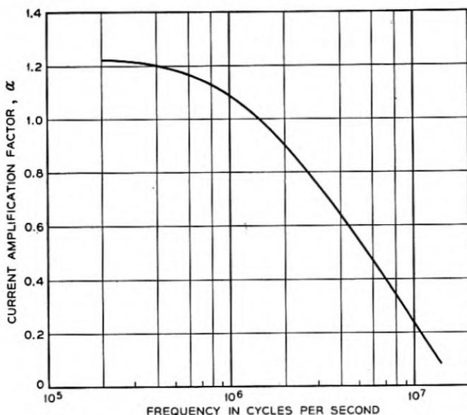
Fig. 12—Current amplification factor  $\alpha$  vs. frequency
