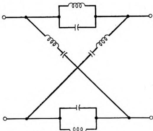
Fig. 2—Basic lattice delay section.
