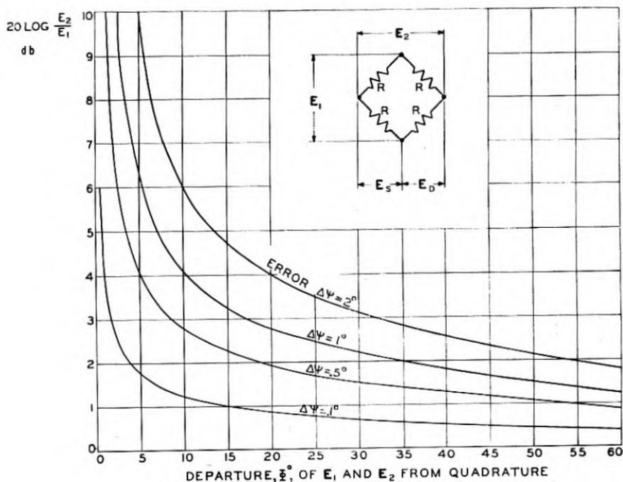
Fig. 8—Phase error  $\Delta\psi$  for unequal inputs.
