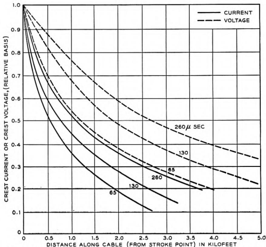
Fig. 5—Variation in crest current in cable and in voltage between sheath and copper shield for stroke currents having various times to half-value as indicated on curves, for an earth resistivity of 1000 meter-ohms.
