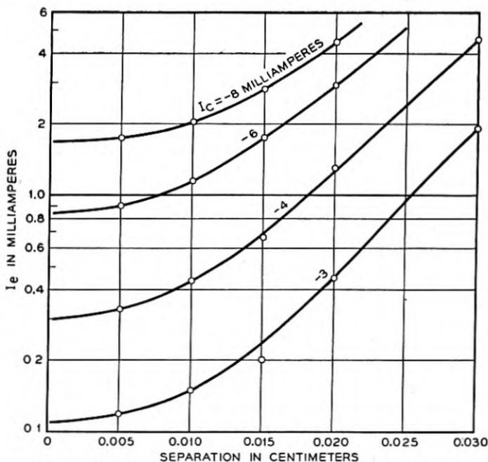
Fig. 8—Emitter current  $I_e$  vs separation for fixed  $I_s$  and  $V_c$ .
