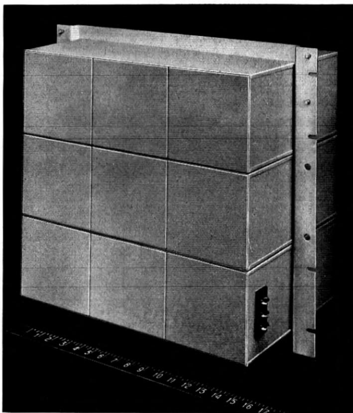
Fig. 13—Exterior view of the band elimination filter.
