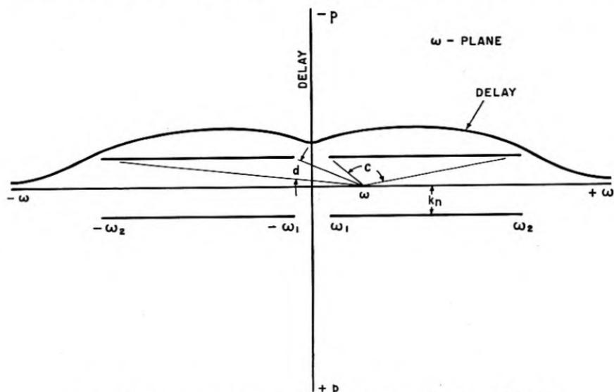
Fig. 6—Delay-frequency characteristic of the network of Fig. 5.
