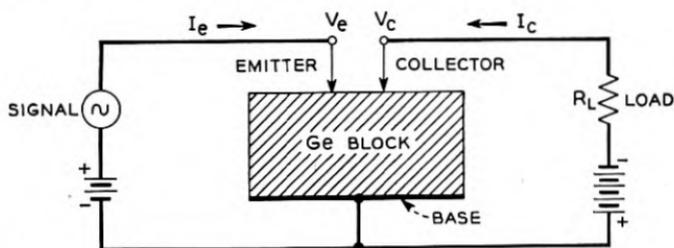
Fig. 1—Schematic of transistor showing circuit for amplification of an a-c. signal and the conventional directions for current flow. Normally  $I_e$  and  $V_e$  are positive,  $I_c$  and  $V_c$  negative.
