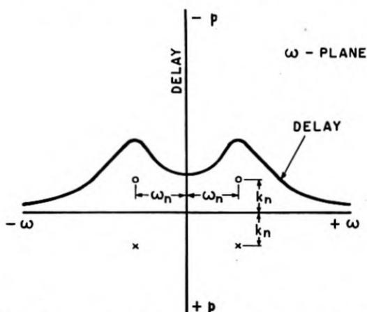
Fig. 4—Delay-frequency characteristic of the network of Fig. 2.
