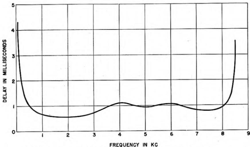
Fig. 1—Unequalized delay distortion of carrier program terminal.
