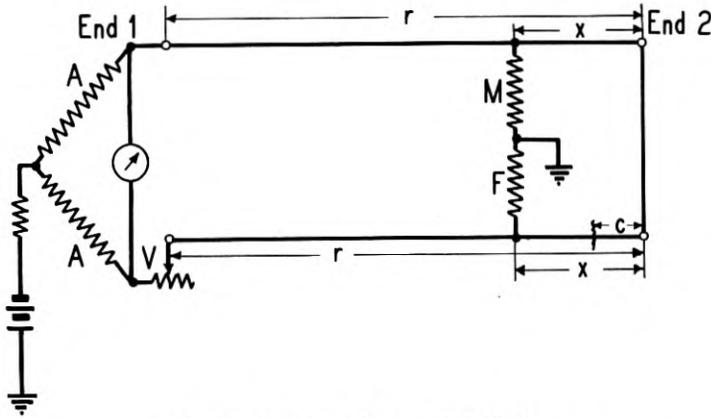
Fig. 10—Location of a resultant fault.
