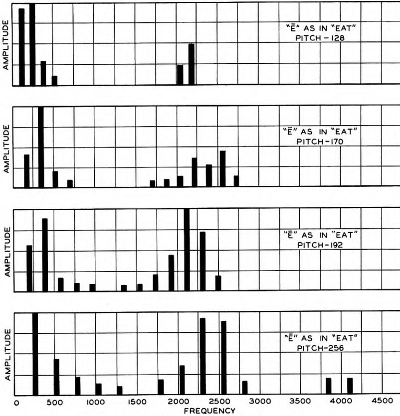
Fig. 9—Spectra of "E" intoned at different pitches.
