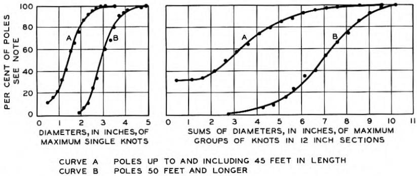
NOTE: "PER CENT OF POLES" REFERS TO THE PER CENT OF POLES HAVING SINGLE KNOTS OR GROUPS OF KNOTS SMALLER THAN THE SIZES INDICATED ON THE BASE LINE. FOR EXAMPLE, 58 PER CENT OF THE POLES 50 FEET AND LONGER HAVE MAXIMUM SINGLE KNOTS SMALLER THAN 3 INCHES IN DIAMETER
