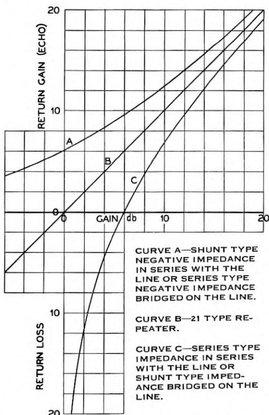
Fig. 12—Echoes caused by boosters and 21-type repeaters.
