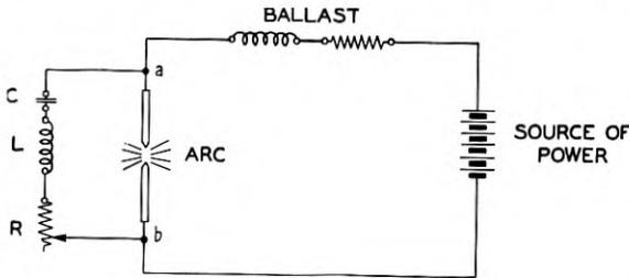
Fig. 6—Arc as a negative resistance.
