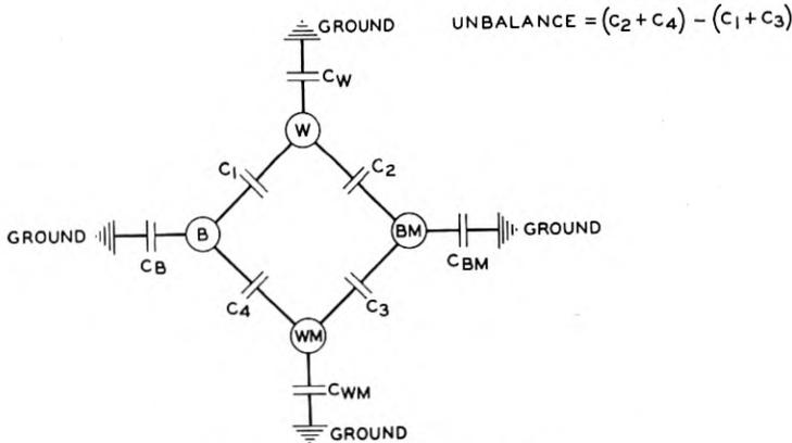
Fig. 37—Side-to-side capacitance unbalances.
