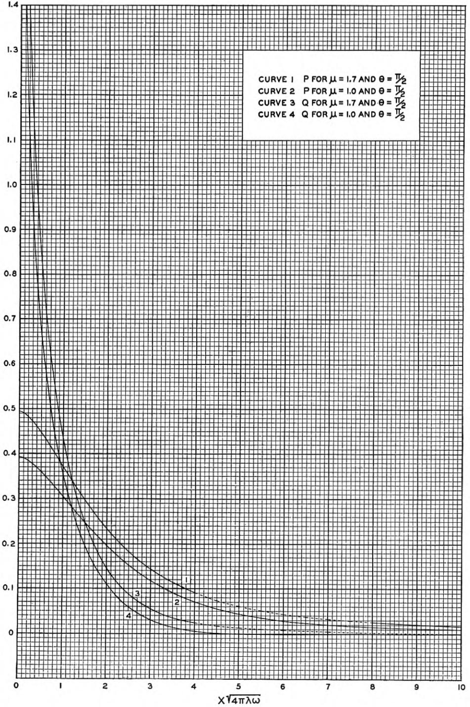
The curves show the effect of  $\mu = 1.7$  on the mutual impedance between two parallel ground return circuits with the wires lying on the ground. The dashed portions of the curves were not computed.
