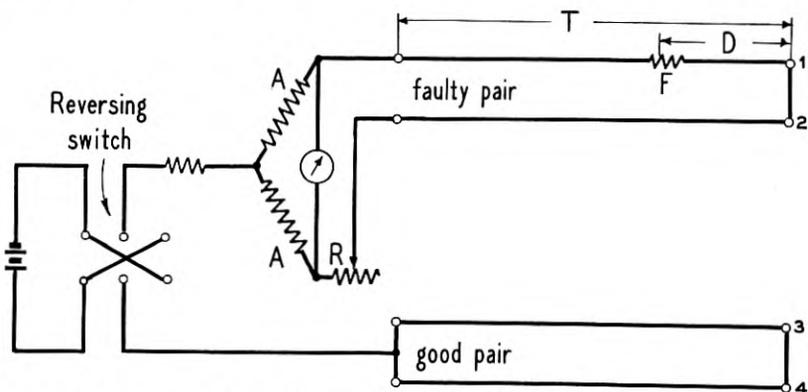
Fig. 14—Schematic circuit—long cable method for locating a series resistance unbalance.
