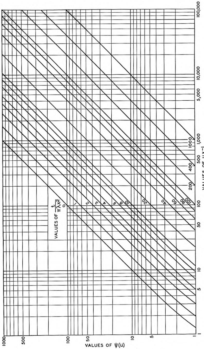
Fig. 3— $\psi(u)$  for a range in which  $\psi(u) \approx 1$ ,  $1 \leq ux^{-1} \leq 100,000$ . The straight line portion of the curve plots the equation
