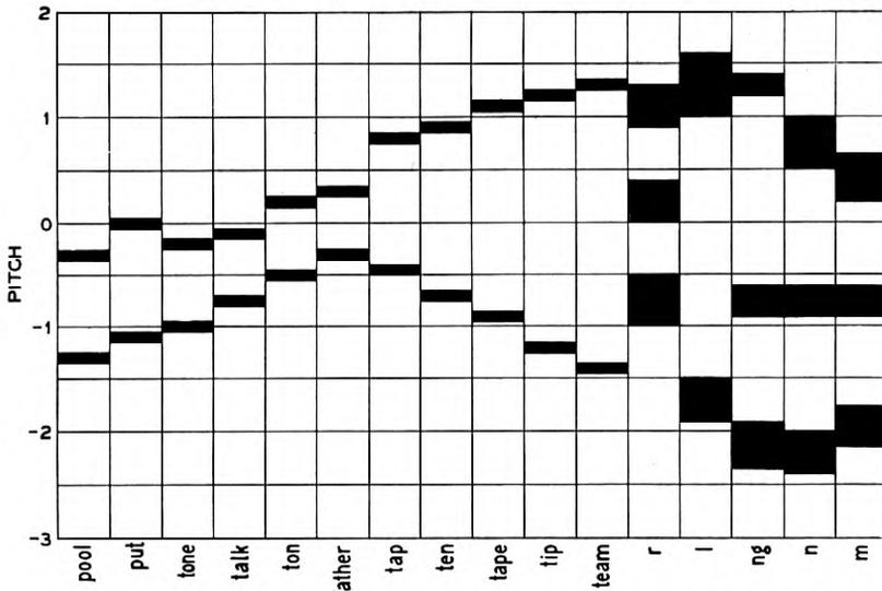
Fig. 10—Characteristic resonance positions for the spoken vowels.
