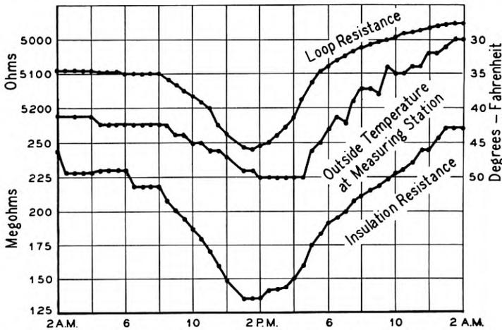
Fig. 3—Variation of insulation resistance, loop resistance and pair temperature over 24 hour period—typical 50 mile aerial cable pair.
