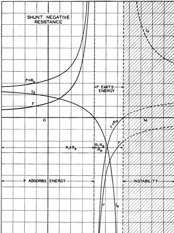
Fig. 5—Curves illustrating properties of shunt negative resistances.
