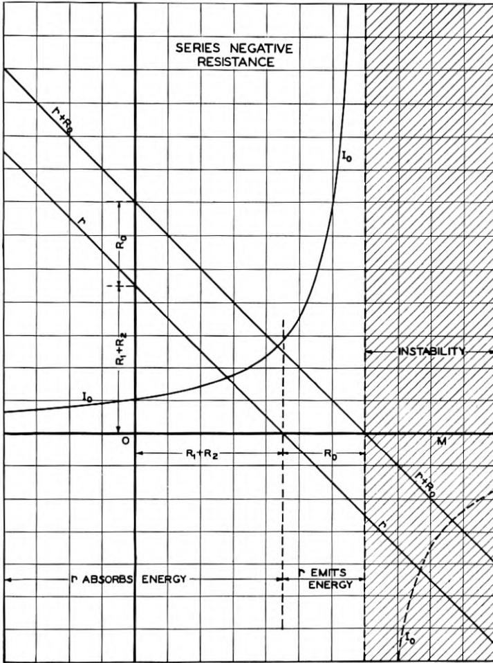
Fig. 3—Curves illustrating properties of series negative resistances.
