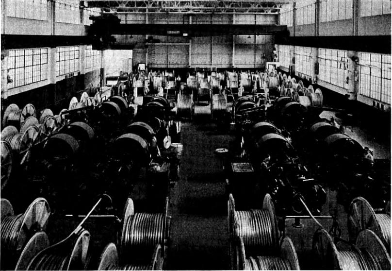
Fig. 40—Tape armoring machine.
