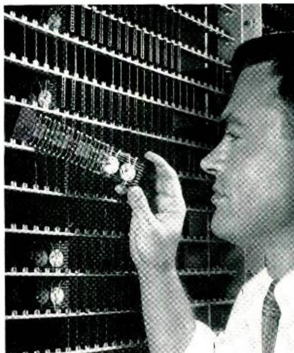
*R. E. Eberhardt, Illinois Bell, on loan to Bell Laboratories, holding a printed-circuit card (two transistors can be seen mounted close to hand). View also shows close spacing of cards in bay.*
