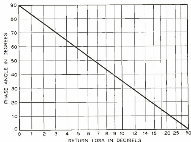
Fig. 5 — Phase angle is proportional to return loss.
