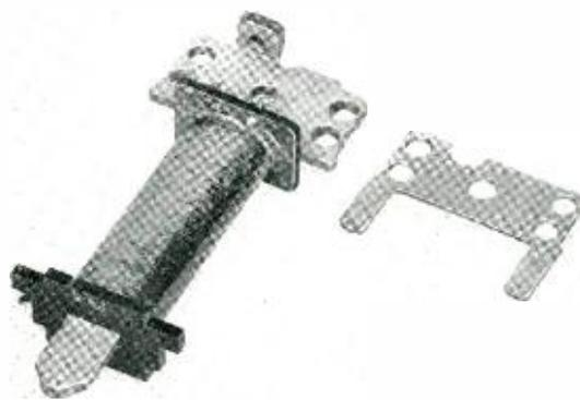
Fig. 3—New EA relay coil assembly, spoolheads with backstop lugs, and the magnetic shunt.
