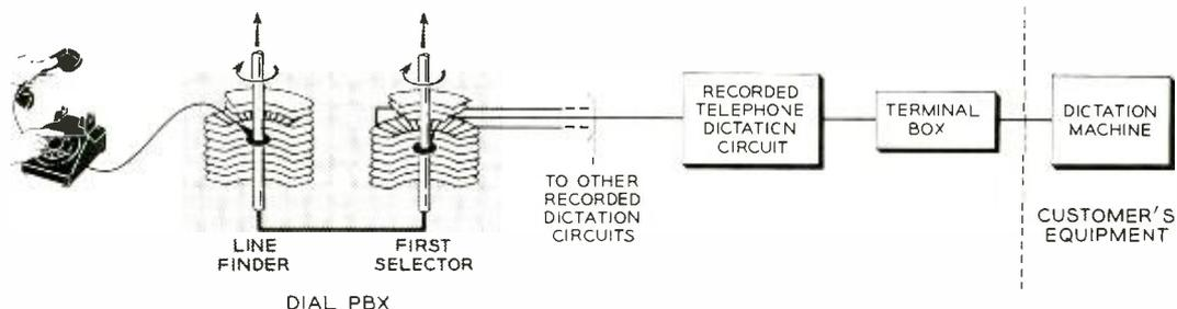
Fig. 2— Each extension has access to the switch level set aside for recorded telephone dictation.
