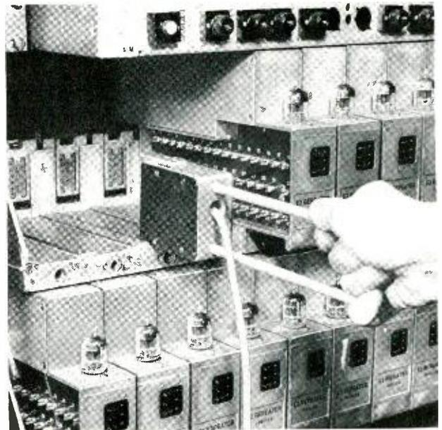
*Fig. 2 — A special plug-in adapter permits the set to be connected in place of the repeater during tests.*
