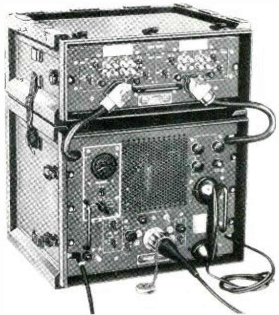
*Fig. 1 — Four-channel modem unit mounted above its associated amplifier-power supply.*
