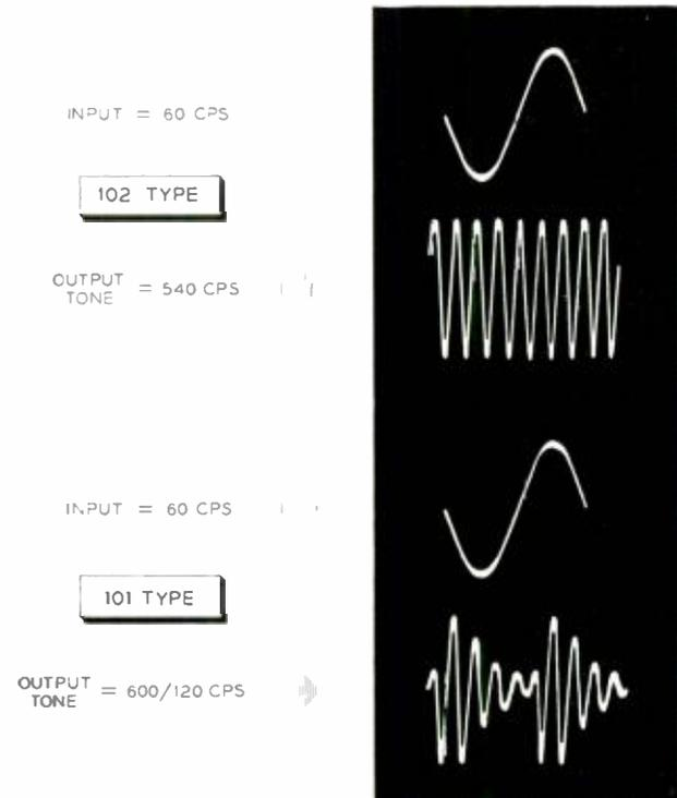
Fig. 2 — Input and output voltages of the 101- and 102-type tone generators for use in small dial offices.
