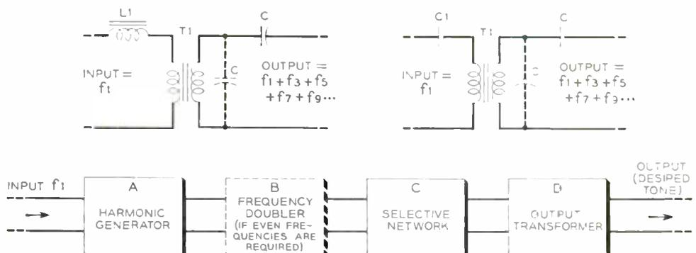
After the harmonic generator (A), a frequency doubler (a rectifier arrangement) circuit (B) is used if it is necessary to convert the odd harmonics to even harmonics. A selective network (C) then filters or shapes the train of harmonics into the
