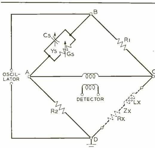
Fig. 2—The basic circuit is that of a Maxwell bridge.
