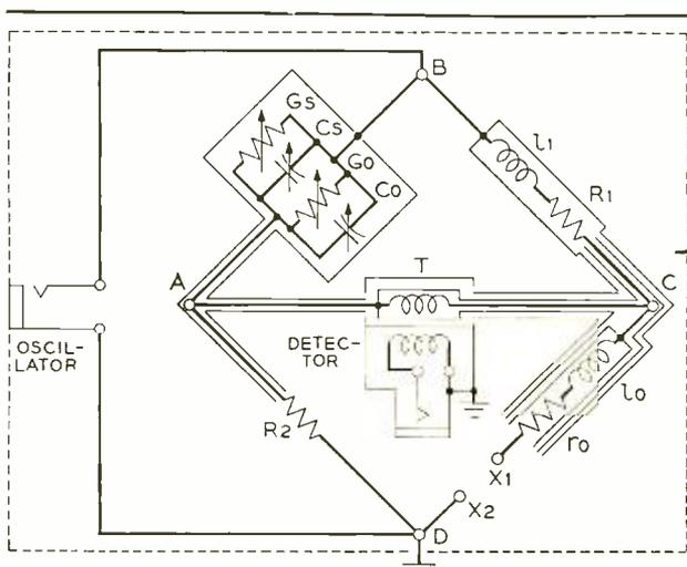
Fig. 3—The complete schematic of the bridge, including the shields.
