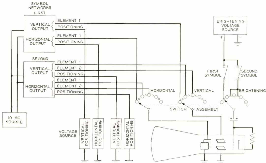
Fig. 8—A simplified diagram illustrating the use of the switch assembly in applying the wave forms for a single and double-element character to the CRO tube.
