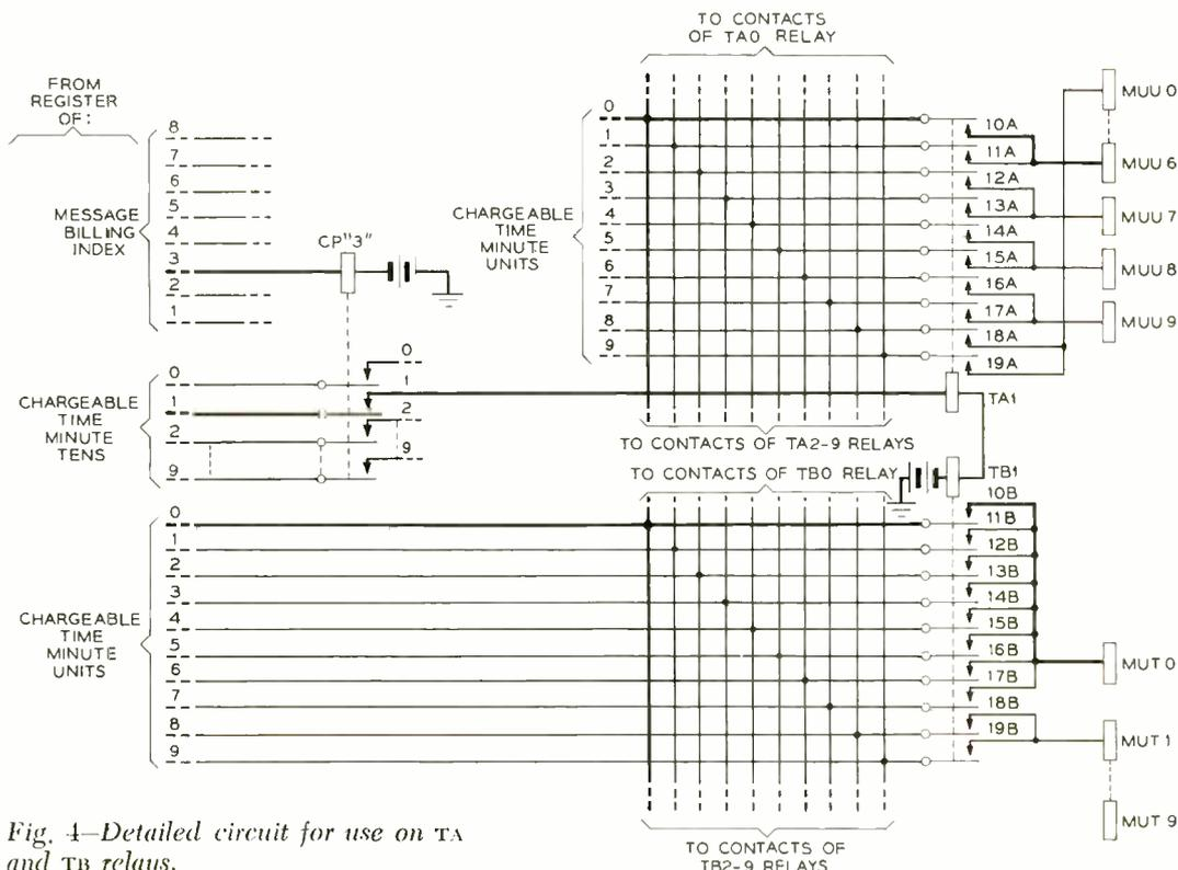
Fig. 4—Detailed circuit for use on TA and TB relays.
