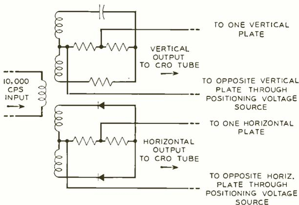
Fig. 4—Simplified schematic for the network used to produce the wave forms for the letter "C". This network is shown at the left of Figure 3.
