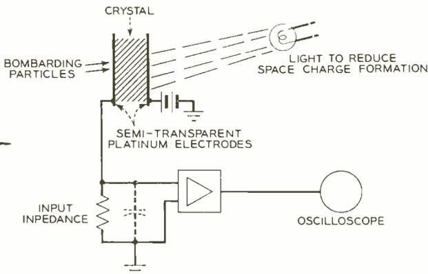
Fig. 2—Typical schematic for studies of bombardment conductivity in insulating crystals.
