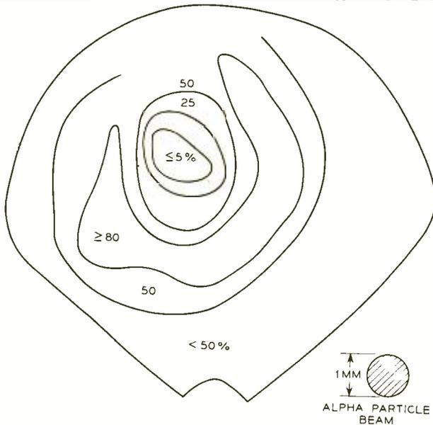
Fig. 6—Plot of the counting efficiency in per cent of a large flat diamond when bombarded by alpha particles. Such wide variations in sensitivity in different parts of a diamond are usually encountered.
