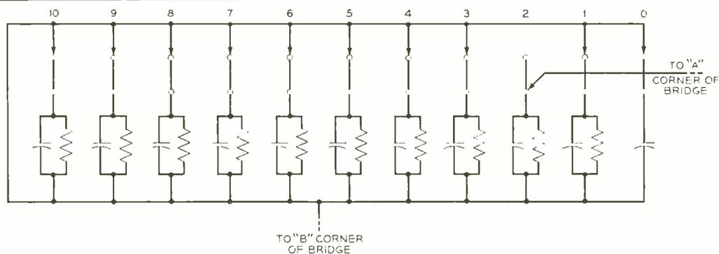
Fig. 4—A developed circuit of the decade conductances. Rotor switches connect all resistance-capacitance networks to ground except one, for each position of the decade dial.
