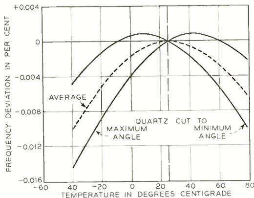
Fig. 3—Temperature characteristics of a typical quartz cut used in repeater oscillators.
