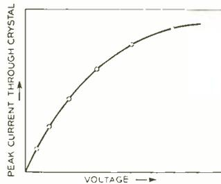
Fig. 3—Variation of electron current through crystal as a function of applied voltage. This is for a diamond crystal bombarded by 10-kilo-volt electrons.
