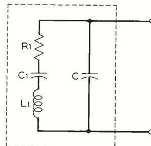
*Fig. 1 — Equivalent electrical circuit of a quartz crystal.*
