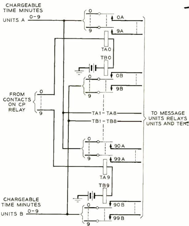
Fig. 3—Schematic showing the arrangement of the TA and TB relays associated with each CP relay.
