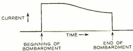
Fig. 4—Electron current flow through a diamond as a result of bombardment by a 10  $\mu$ -second pulse of 10-kilovolt electrons. The decrease in current near the end of the pulse is caused by the formation of an internal space charge field during the period of the bombardment.
