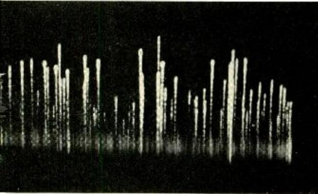
Fig. 5—Pulses from a diamond crystal bombarded by monoenergetic alpha particles. Observe the scatter in pulse heights due to nonuniform response.
