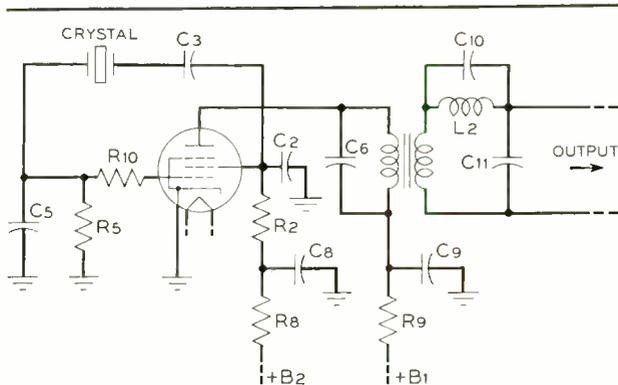
Fig. 2—Circuit of the 304 kc (group unit and repeater) oscillator.
