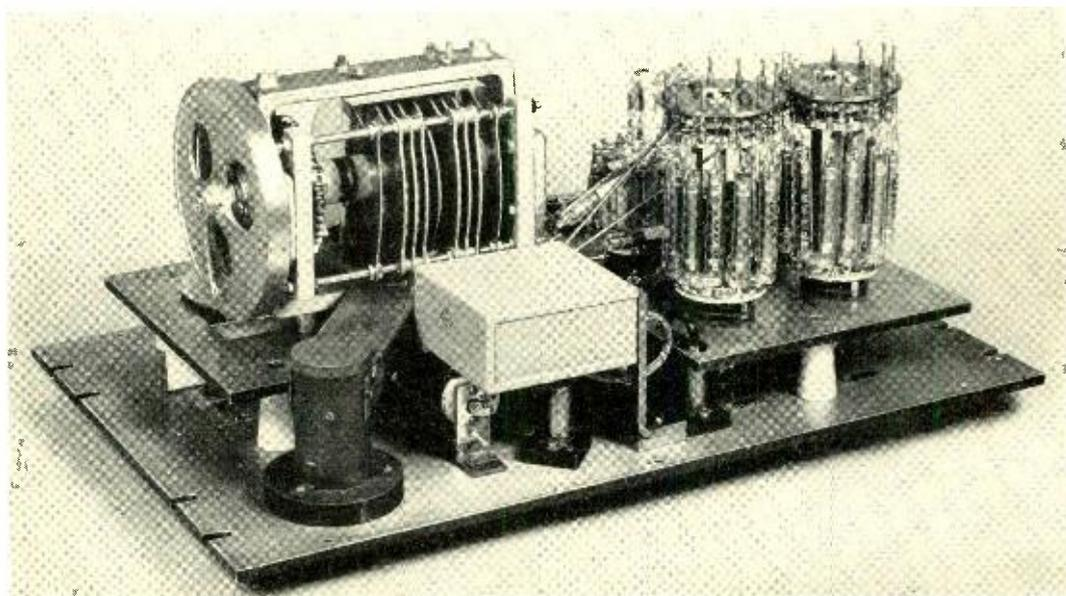
Fig. 1—Interior of the bridge. Standard capacitor  $C_s$  is on the left and decade conductances  $G_s$  on the right.
