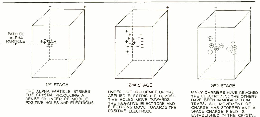
Fig. 1—Simplest case of alpha bombardment conductivity.
