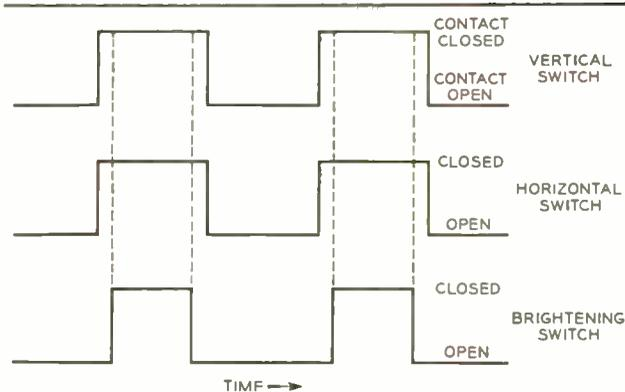
Fig. 7—A diagram showing the magnitude and time relationship of the open and close times of the horizontal, vertical, and brightening switches.
