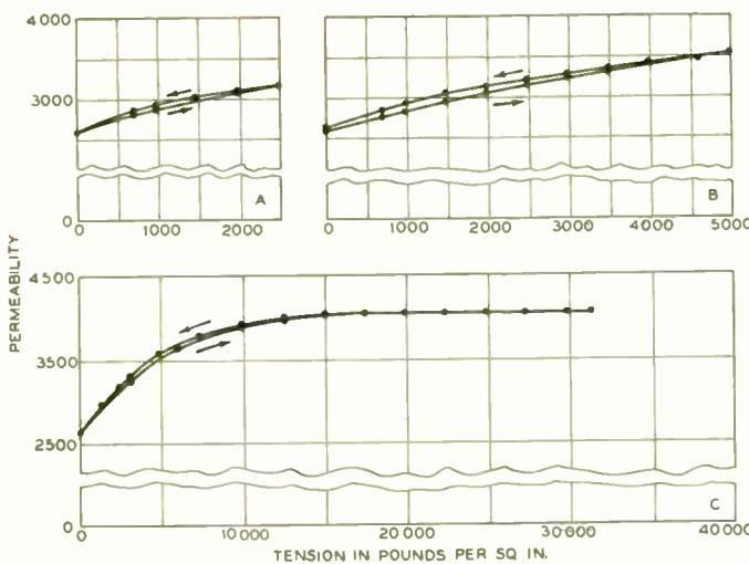
*Fig. 6—Variation of permeability with tension of a permivar tape with a d-c magnetizing force of 3.5 oersteds*
