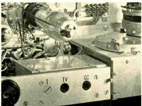
*Fig. 2—Front of the type-K amplifier showing hole for the 554A tool, and the index line marked on a small metal clip, which is attached in the proper position during the factory test*
