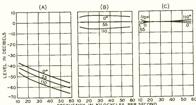
*Fig. 7—Level frequency characteristic of carrier currents after passing over one section of line, at A; the effect of line amplification and line equalizer, at B; the effect of flat-gain regulation, at C*
