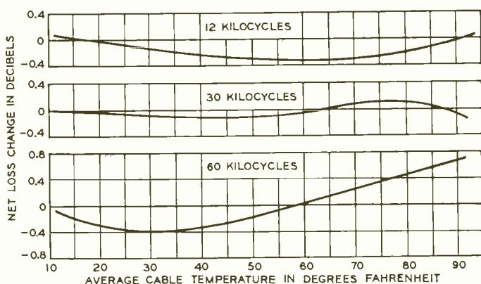
*Fig. 8—Overall performance of the type-K carrier telephone system for a one-hundred-and-fifty-mile circuit*
