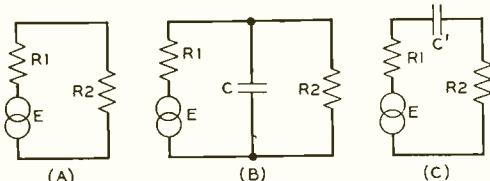
Fig. 2—Equivalent networks of one stage. (A) mid-band; (B) at high frequencies; (C) at low frequencies;  $R_1$  is the parallel resistance of the tube and the plate resistor;  $R_2$  resistance of the grid circuit of the succeeding tube;  $C$ , total shunt capacity;  $C'$  coupling condensers;  $E$ , voltage or equivalent plate-circuit generator
