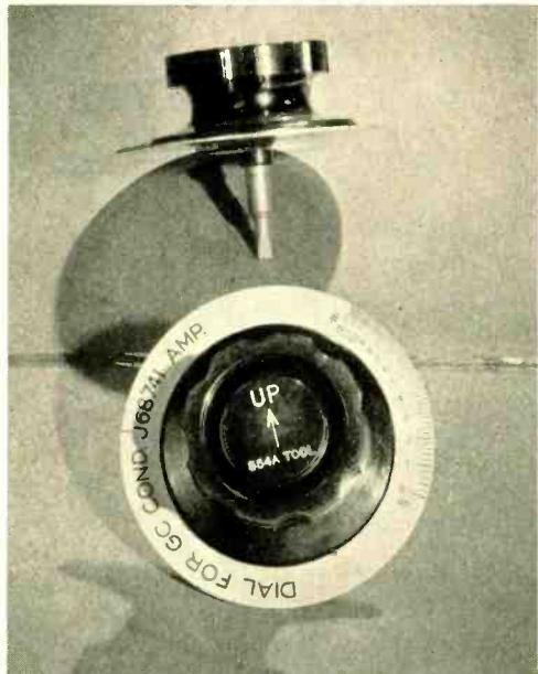
*Fig. 1—The 554A tool photographed in front of a mirror so as to show the rear of the tool and the screw-driver tip, as well as the front and dial carrying a db scale*
