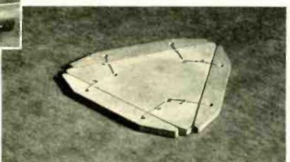
Fig. 4 (right)—Lavite form used for forming and heat treating magnetic specimens
