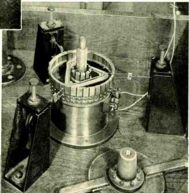
Fig. 2 (right)—Arrangement of permeameter with respect to the three tension wires attached to frame
