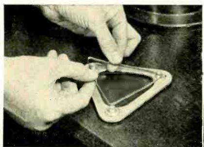
Fig. 1 (left)—A triangular frame with sliding pins in each corner is used to apply tension to the magnetic specimen
