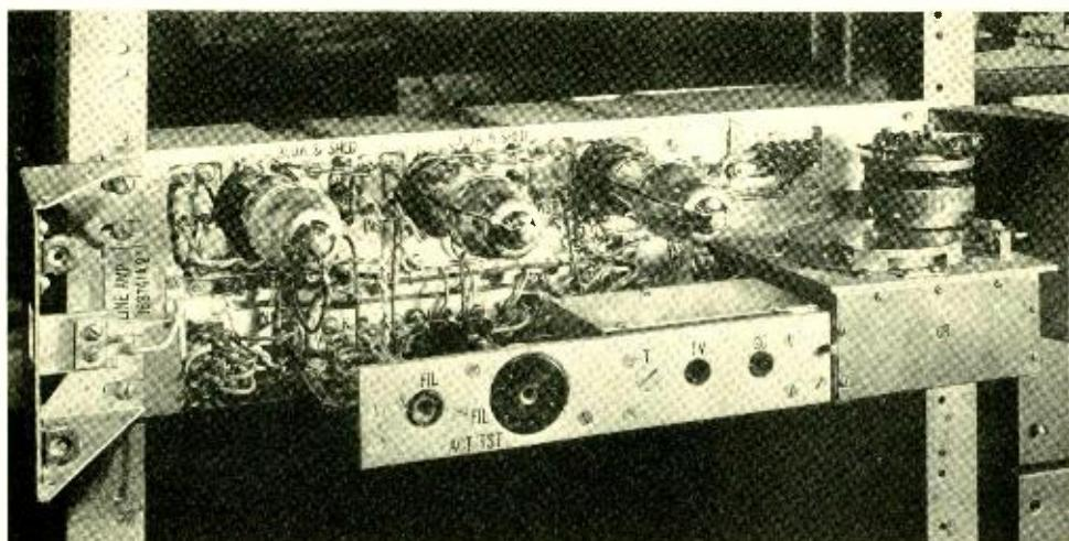
Fig. 1—Amplifier for the type-K carrier system with cover removed
