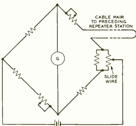
Fig. 3—A Wheatstone bridge circuit is employed to determine the mean temperature of a section of cable—a pilot pair in the cable serving as one arm of the bridge
