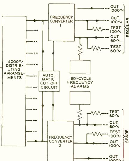
Fig. 1—Simplified block schematic of the system for supplying reference frequencies
