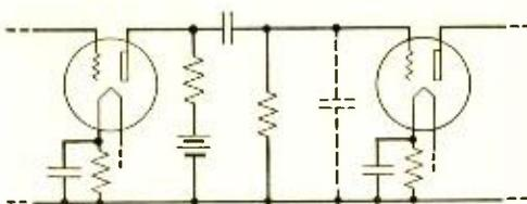
Fig. 1—Simplified schematic of a typical resistance-coupled amplifier
