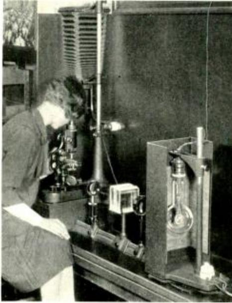
*Miss Marshall adjusts the microscope before photographing a timber section*
