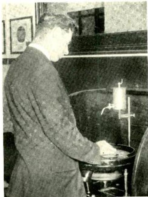
*R. R. Ziegler puts the final polish on a steel specimen*
