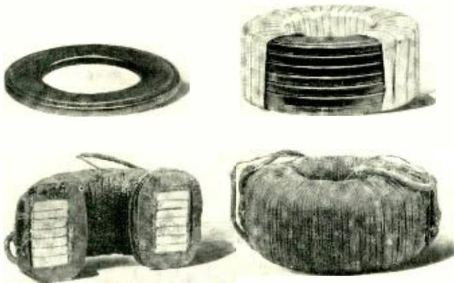
Fig. 2—Loading coil with compressed powdered core: top, left—core ring, right—partially taped core; bottom, left—coil sectioned, right—coil ready for potting
