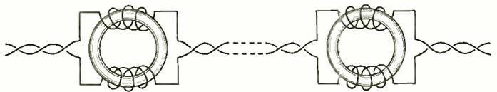
Fig. 1—Method of connecting loading coils into cable pair
