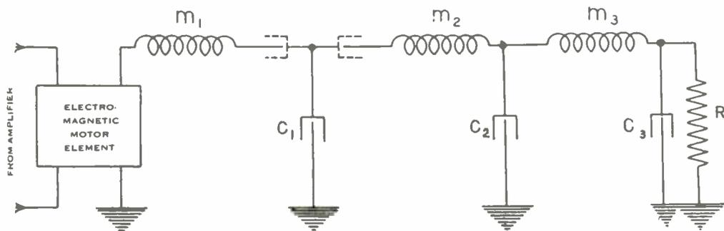
*Fig. 2. Schematic of Electrical System Analogous to Recorder*
