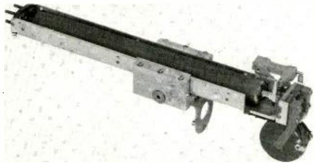
*An up-side-down view of the "rubber line" recorder*
