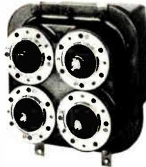
Designed to switch two transmitters from antenna to dummy load, the 6730E interfaces with 1 5/8 inch coaxial cable. For 3 1/8" lines, the 6740-B transfer switch is used. Either manually or remote controlled, the **Transfer Switch** is fully interlocked and can be wired to existing equipment to prevent "hot" switching.
