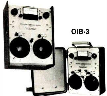
The **Operating Impedance Bridge** measures the impedance of networks, radiators, and the like while they operate under full power. VSWR as well as complex impedances of up to  $400 \pm j300$  ohms can be measured.
