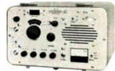
The **Receiver/Generator** combines a two-watt RF output and a correlation detector circuit that virtually eliminates interference problems. The RG-3 can be used in conjunction with any conventional impedance bridge including the OIB series.
