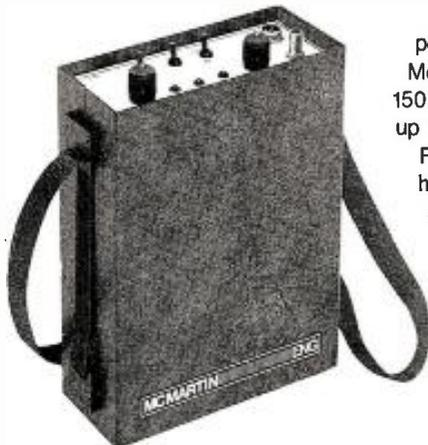
It's 3 watts, six pounds and very portable. Report in first with the new McMartin RPU-1103, a self-contained 150 MHz battery-operated, remote pick-up transmitter. It exceeds all the latest F.C.C. requirements. The RPU-1103 has dual frequency operation and an audio compressor that functions on both line (portable cassettes, etc.) and microphone inputs to allow simple talk over operation. This ENG machine is the latest addition to the McMartin broadcast line.
