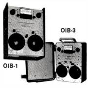
The Operating Impedance Bridge measures the impedance of networks, radiators, and the like while they operate under full power. VSWR as well as complex impedances of up to 400 ± j300 ohms can be measured.
