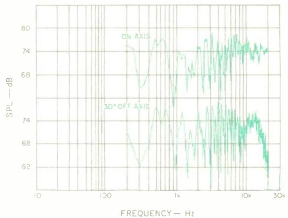
**Fig. 6—**Three-meter room response measured on axis and 30° off axis; off-axis curve has been lowered for clarity.
