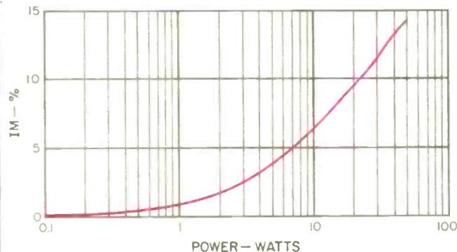
**Fig. 15—IM produced by mixing  $A_4$  and  $E_1$  in equal proportion.**
