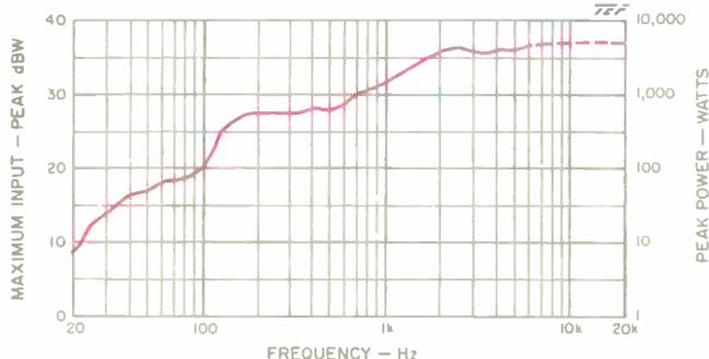
**Fig. 18—Maximum peak-input power for moderately clean output. Above about 6 kHz (dashed portion of curve), limitations are imposed by clipping of 5.5-kilowatt amplifier, not by the speaker. Input signal was a shaped tone burst; see text.**
