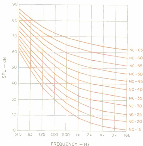
**Fig. 6—Background-noise criteria curves. The NC-30 curve is the maximum allowable in a THX theater; NC-25 is recommended where practical (after Beranek).**
