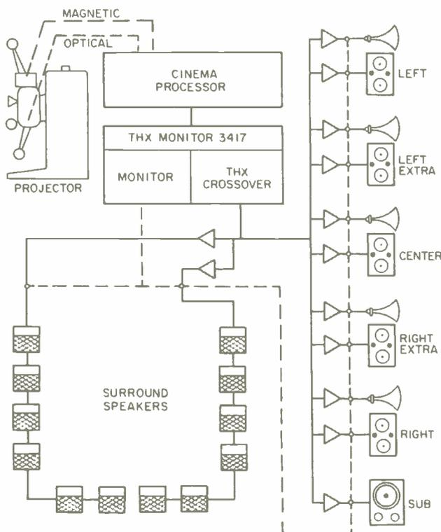
**Fig. 1—Block diagram of typical 70/35-mm THX Sound System. Theaters using only 35 mm do not require the "Left Extra" and "Right Extra" screen speakers.**
