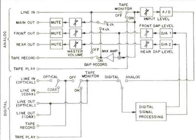
**Fig. 1—Block diagram of one set of channels (left or right) of the XP-A1010 processor.**
