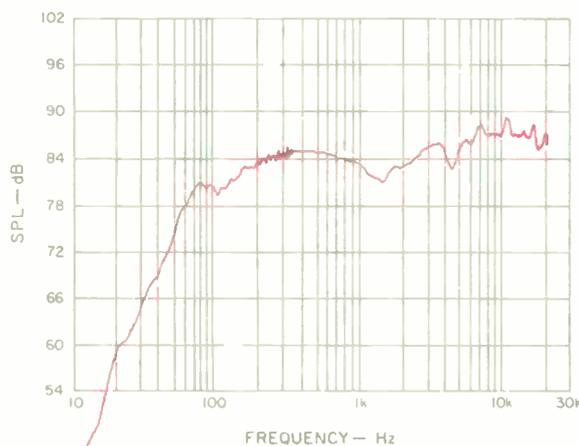
**Fig. 3—One-meter on-axis anechoic frequency response with an input of 1 watt into 4 ohms (2.0 V).**
