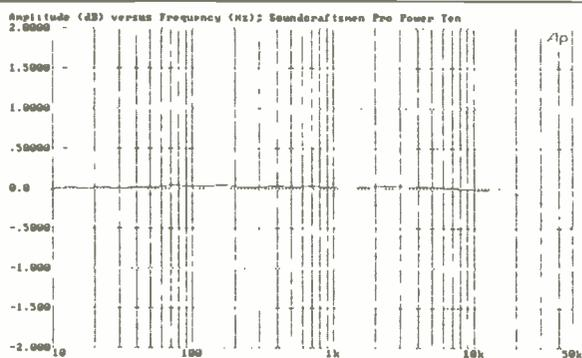
**Fig. 1—Frequency response of the Soundcraftsmen Pro-Power Ten amplifier.**
