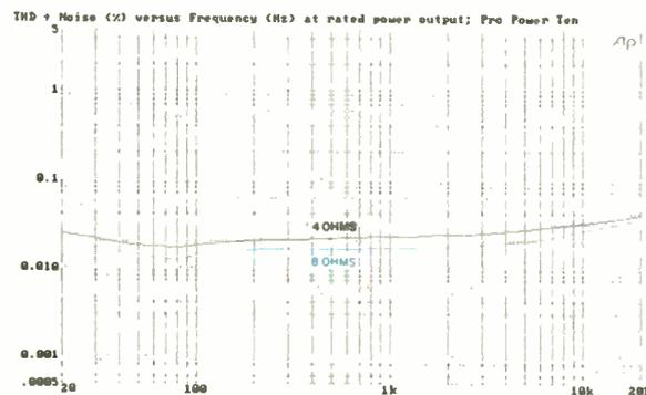
**Fig. 4—THD + N vs. frequency, at rated power, for 8- and 4-ohm loads.**
