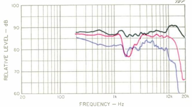
**Fig. 9—Mean vertical on- and off-axis frequency response curves. Top curve is mean on-axis curve, an average of response measurements made within  $\pm 15^\circ$  of vertical and horizontal axes. Middle curve is average of measurements**
