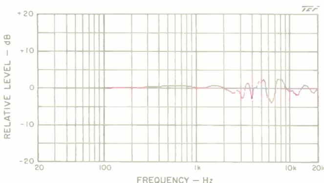
**Fig. 5—Effect of grille on axial 1-meter frequency response. (The graph is normalized to show only differences from grille-off response of Fig. 1.) The grille adds fairly severe response aberrations in the range from 3 to 10 kHz.**
