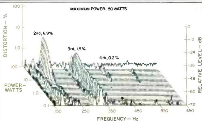
**Fig. 13—Harmonic distortion for the musical tone  $A_2$  (110 Hz). The second and third harmonics were the only significant ones in this power range. Note the rapid increase in second harmonic at power levels above 10 watts; see text.**
