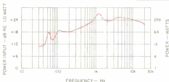
**Fig. 13—Power linearity (input power handling vs. frequency for 1 dB compression of the output).**
