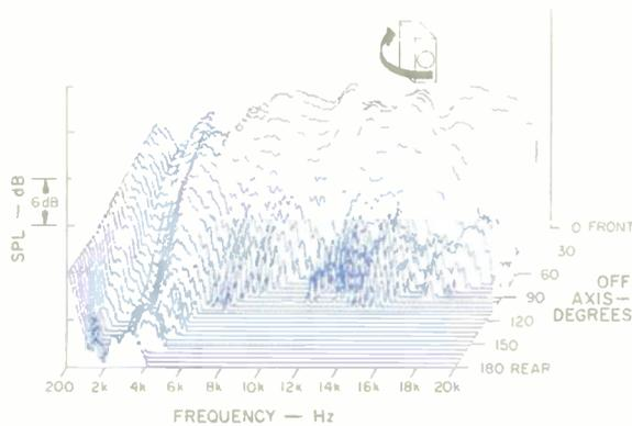
**Fig. 7—**Horizontal off-axis response plots taken from the front, around the side, to the rear of speaker.
