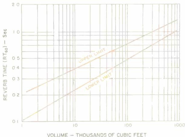
Fig. 5—Upper and lower reverberation-time ( $RT_{60}$ ) limits for THX theaters of various volumes, at 500 Hz.
