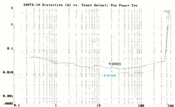
**Fig. 5—SMPTE-IM distortion vs. power output for 8- and 4-ohm loads.**
