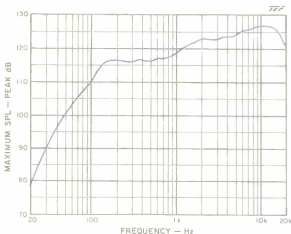
**Fig. 19—Maximum peak SPL output at 1 meter, on axis, for input levels shown in Fig. 18. The system can generate peak levels in excess of 115 dB SPL above 150 Hz.**
