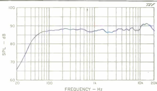
**Fig. 1—One-meter on-axis frequency response, with an input of 2.83 V rms (equivalent to 1 watt into the rated 8-ohm impedance).**
