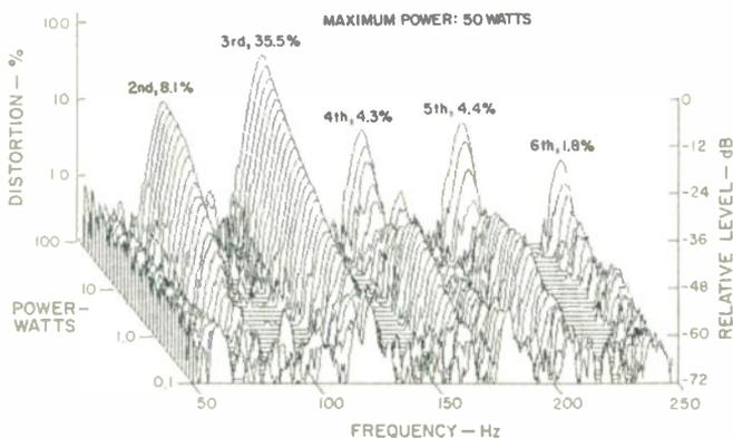
**Fig. 12—Harmonic distortion for the musical tone E<sub>1</sub> (41.2 Hz).** Note relatively high third-harmonic level at high powers; see text.
