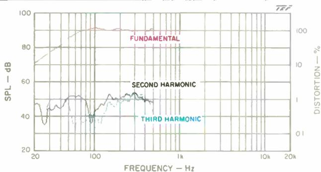
**Fig. 16—Second- and third-harmonic distortion levels vs. frequency for 90 dB SPL mid-band output at 1 meter on axis; input signal is 3.6 V rms (1.6 watts into 8 ohms).**
