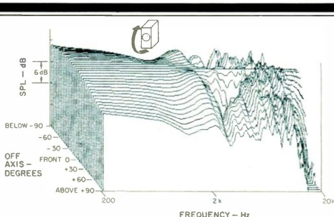
**Fig. 7—Vertical off-axis plots taken from above to below the system. Note log frequency scale and normalization of all curves to the on-axis response. Also note crossover response irregularities between 1.5 and 3 kHz, at roughly 20° to 40° off axis up and down.**
