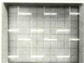
**Transmission characteristics for 15 ft. of WeberWire—1 source, 8 resistive load—communicating a 100 kHz square wave.** The upper limit of WeberWire is just beginning to be observed as the extremely high harmonics of the overshoot from the signal generator are noticeably reduced.
