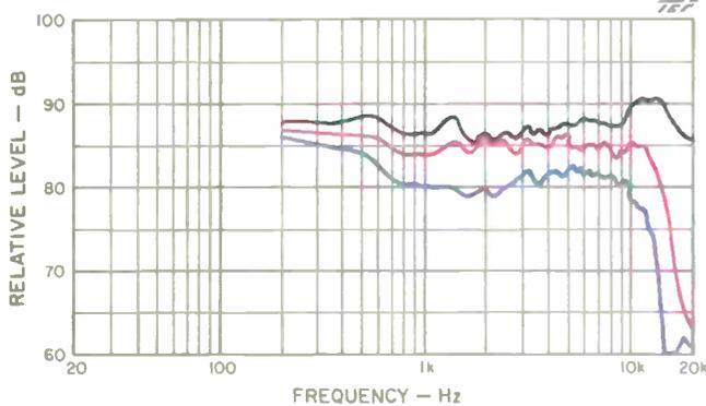
**Fig. 8—Mean horizontal on- and off-axis frequency response curves above 200 Hz; see text. Top curve is mean on-axis curve, an average of response measurements made within  $\pm 15^\circ$  of vertical and horizontal axes. Middle curve is**
