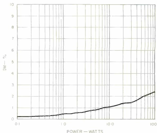
**Fig. 12—IM produced by mixing A<sub>4</sub> and E<sub>1</sub> (440 and 41.2 Hz) in equal proportion.**
