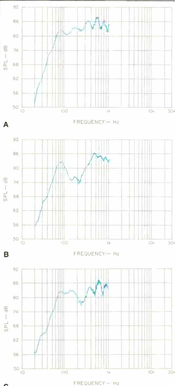
**Fig. 4—Effect on system amplitude below 1 kHz of placing low-frequency module at same distance from microphone as satellite (A), 24 inches closer than satellite (B), and 24 inches farther than satellite (C). At the 140-Hz crossover frequency, 24 inches is  $\frac{1}{4}$  wavelength.**
