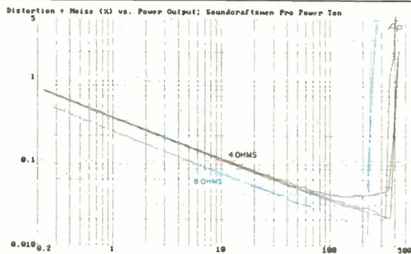
**Fig. 3—THD + N vs. power output into 8- and 4-ohm loads. Just before curves slope upward, top curve is 20 kHz, straightest curve is 1 kHz, and remaining curve is 20 Hz.**
