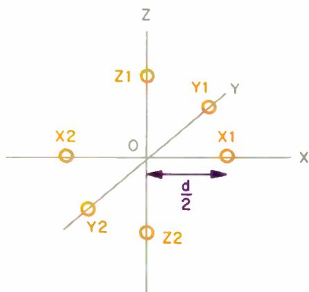
**Fig. 2—Two-dimensional representation of the three-dimensional array of measurement microphones used in developing the XP-A1010. The "Y" axis, shown here as a diagonal, would actually be at right angles to this page; see text.**
