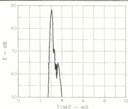
**Fig. 4—One-meter on-axis ETC for test signal swept from 200 Hz to 10 kHz. In this range, most of the response shown is from the tweeter.**
