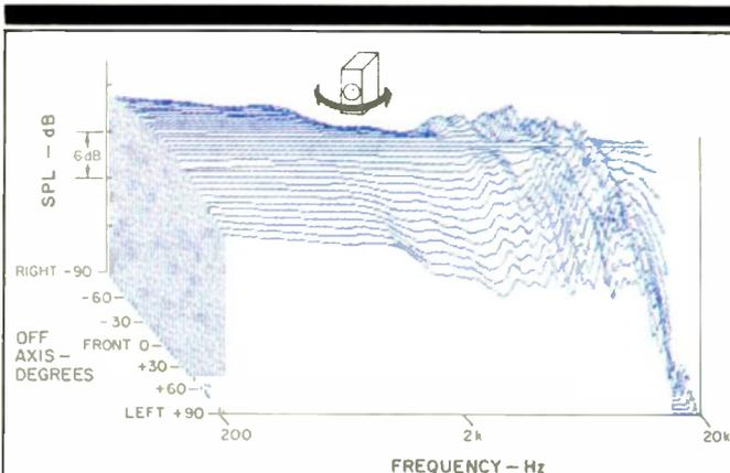
**Fig. 6—Horizontal off-axis response plots taken from the left side, around the front, to the right side of the system. Note that frequencies are shown on a log scale and that all curves are normalized to show differences from the on-axis response.**
