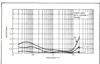
Fig. 6—Distortion versus frequency at various power levels
