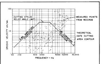
Fig.2—Scatter diagram of "difficult-to-track passages" from commercial records.
