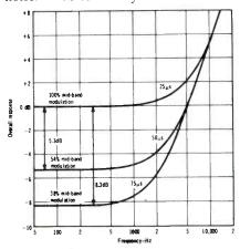
Fig. 1—FM pre-emphasis curves arranged to show maximum permissible mid-band modulation levels with 75  $\mu$ S, 50  $\mu$ S, and 25  $\mu$ S time-constants assuming same net boost (resulting in approximately full modulation) at 10 kHz in all cases.
