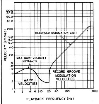
Fig. 5—Extended low frequency trackability requirements.
