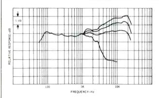
Fig. 2—Range of the continuously variable treble control.
