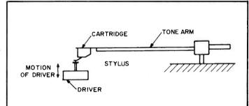
Fig.6—Method for measuring tone arm-cartridge resonance.
