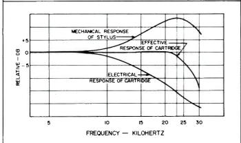
Fig. 12—V15-III frequency response characteristics.
