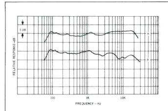
Fig. 1—Response with one-third octave pink noise. Curve A was measured on axis and B was a 45 degrees off axis.
