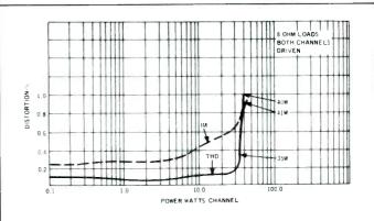
Fig. 5-Distortion characteristics at 1 kHz
