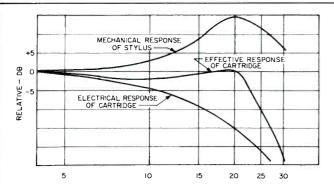
Fig. 11—V15-II frequency response characteristics
