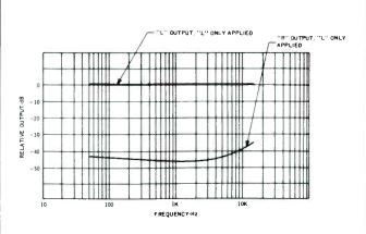
Fig. 6—FM stereo separation characteristics.
