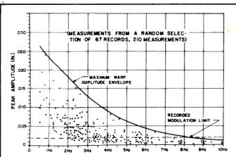
**Fig. 4**—Scatter diagram of warp amplitude and frequency found on commercial records.
