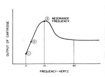
Fig. 7—Output of cartridge as drive frequency is changed near tone arm-cartridge resonance.
