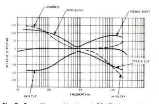
Fig. 8—Tone, filter, and loudness (-30 dB) characteristics.
