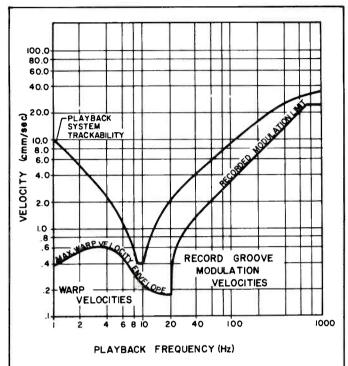
Fig. 8—Typical tone arm-cartridge trackability curve.
