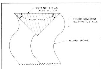
Fig. 1—Top view of cutting stylus in record groove.
