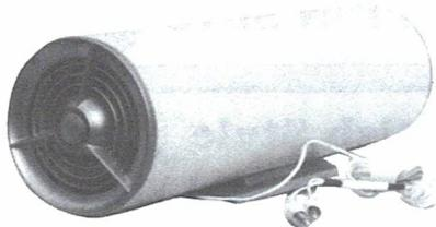
**TRANSISTOR RADIO EXTENSION SPEAKER** – This Japanese-made unit is 12" long and 13" in diameter. The body is made of heavy paperboard tubing with two plastic grilles on both ends. The speaker is mounted two-thirds of the way in. (*Doug Burskey - Mansfield, OH*)
