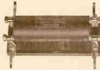
Radio Frequency Transformer Mounted
