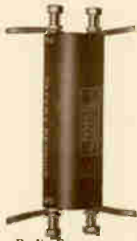
Radio Frequency Transformer
