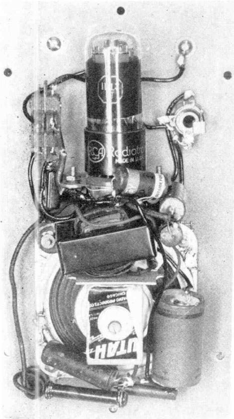
Interior view, showing midget permanent magnet loud-speaker and essential components.
