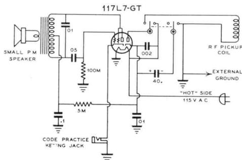
Wiring diagram of combination c.w. keying monitor and code practice oscillator for operation from 110-volt a.c. line.
