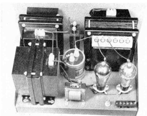
Power supply and filter for final r-f amplifier stage.
