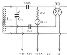
The wiring diagram for a simple grid-dip meter for battery operation.
