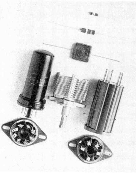
Here are the components (crystal excepted) for the new Wells Oscillator. No simpler oscillator assembly has ever been devised.
