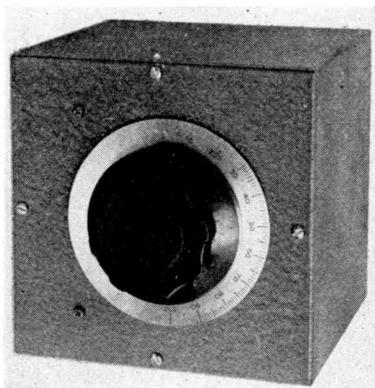
Front view of the 10-meter converter. A vernier tuning dial is a convenience for covering the congested band.
