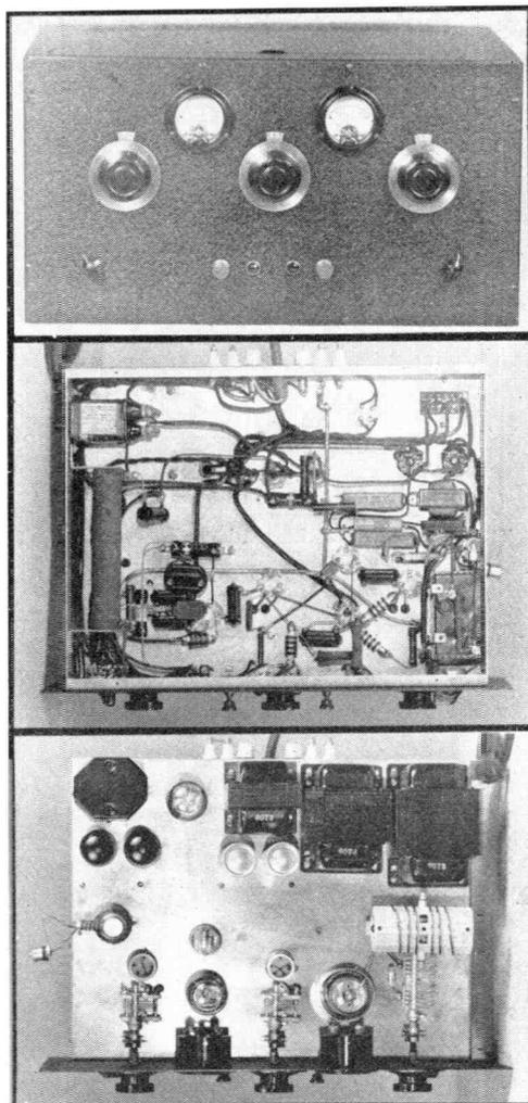
• Three views of the professionally-appearing 'phone transmitter for 10-meter operation, built entirely by Ella. The YLs are giving many an OM something to think about when it comes to transmitter construction.
