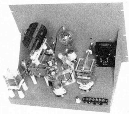
Another 75T r-f amplifier for a cathode-modulated transmitter previously built.
