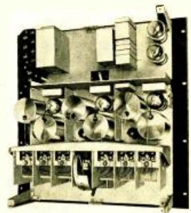
Fig. 2. The famous Western Electric "10-A" tuner which is similar in circuit details and performance to the "MB-30" unit shown in Fig. 1.
