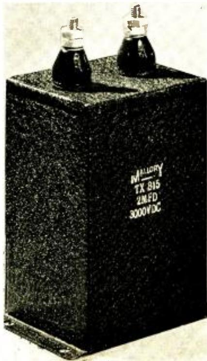
two years of research. The compound is not a wax nor is it like any of the standard or special-named impregnating oils now offered. It does not contain chlorine, and does not depend on chlorination generally used to develop the high dielectric constant necessary for condensers of compact construction. The natural high dielectric constant of Mallory Compound is combined with unusual resistance to heat, thereby providing a good power factor and an extremely stable d.c. resistance. ALL-WAVE RADIO.
