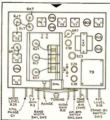
Fig. 2.—Chassis layout for the "One Stop" super.
