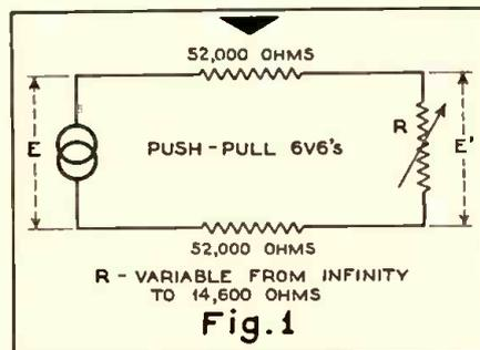
Explanatory diagram which is the equivalent circuit of the driver stage.
