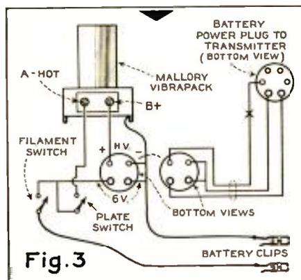
The Vibrapack connections and the connecting plug and cable. Separate plate and filament switches are provided.
