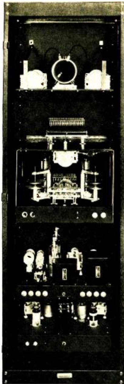
Rear view of the rack containing the r.f. equipment. From bottom to top are: exciter, driver, Class C stage, and antenna tuning unit.
