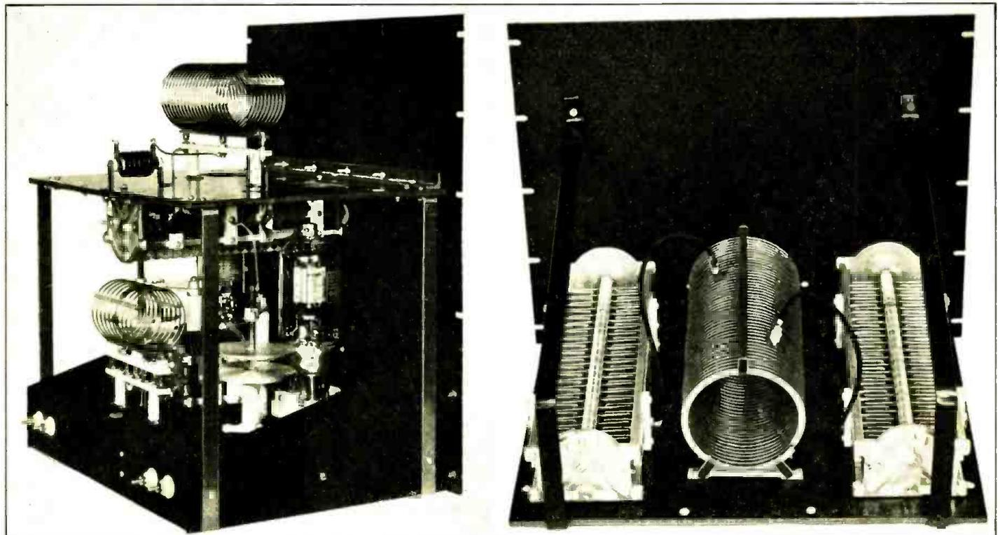
At the left is the Class C final amplifier stage. The antenna tuning unit is shown at the right.
