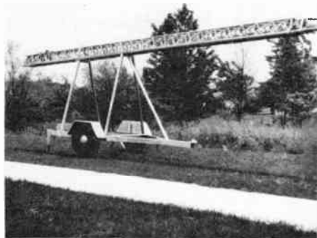
Trailer and Telescoping Tower
