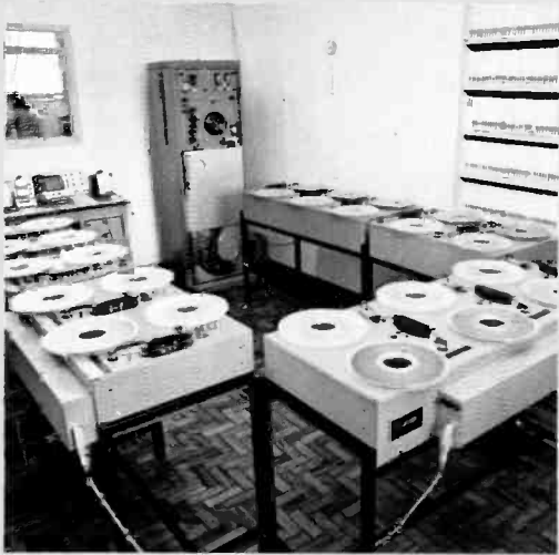
The cassette division is comprised by several operations. The most important of which is that of duplication, since pre-recorded tapes play an important role in the record industry.
