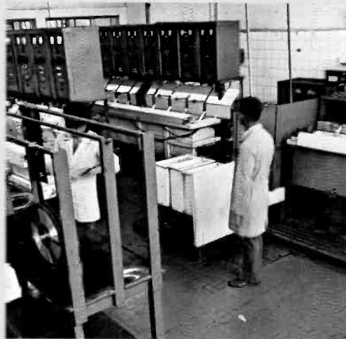
The preparation of lacquers, stampers, and mothers are made in self-built machinery. The total work time is about one hour therefore giving the best quality in the minimum time possible.
