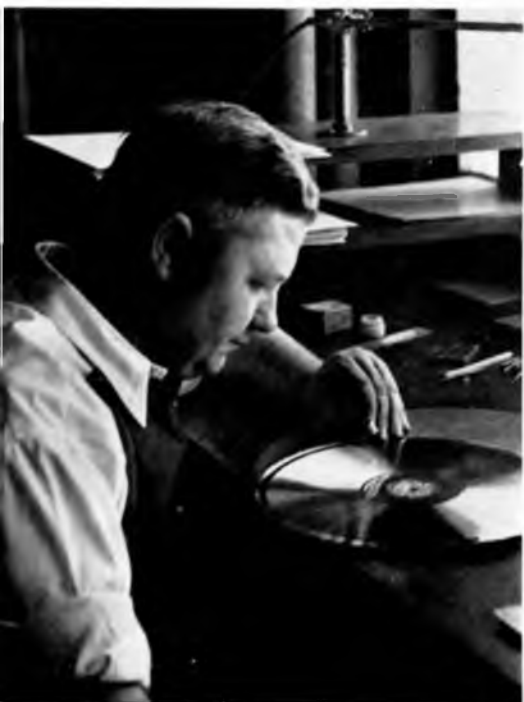
The trimmed and polished matrix is inspected for possible flaws in the grooves with a magnifying glass. Minor repairs are done on spot
