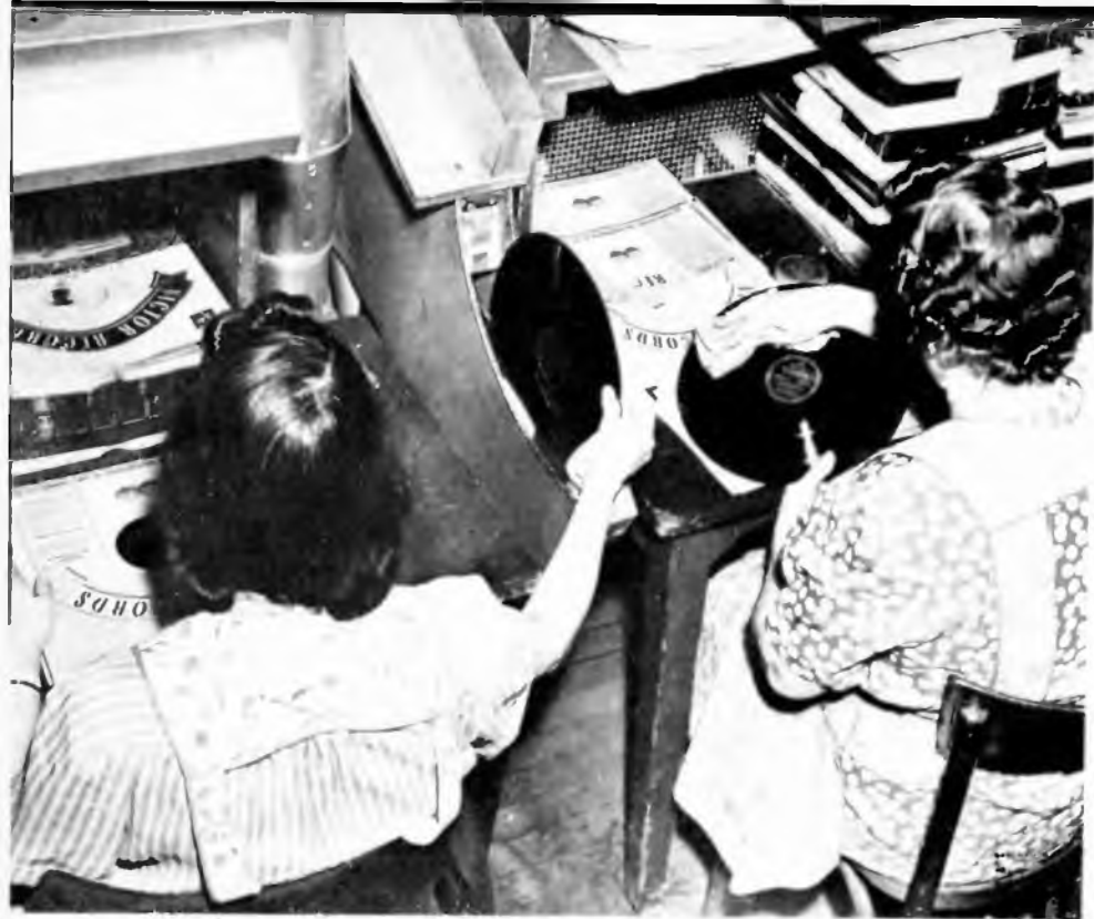
As records come down from edging machine they are put into envelopes, and, having passed test, are sent to shipping department
