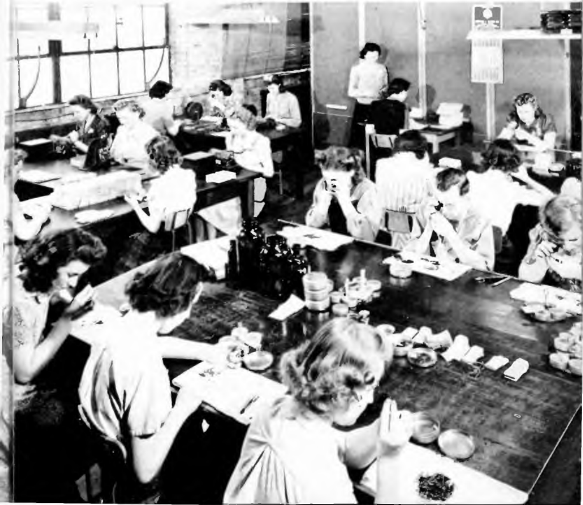
Skilled workers at the Pfanstiehl Chemical Co. (below) examine needles for any flaws. Imperfect needles are discarded quickly.
