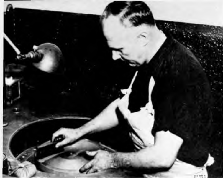
The disc in front of the gold sputtering chamber (other page) is being groomed for the future master print. Next, in the process of transformation from wax to record the disc is coated with an even layer of bronze powder, later to be replaced by silver
