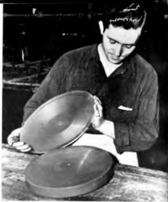
The copper plate, called "master," is pried off the wax disc. Later on it will be nickel plated and a test record will be pressed from it
