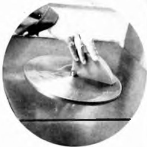
Left: Fred Maisch, Victor's recording engineer, reigns in solitary splendor over the control board. Right: The original record, wax on glass, is prepared to receive the grooves which are cut by the stylus as result of the recording done in the studio
