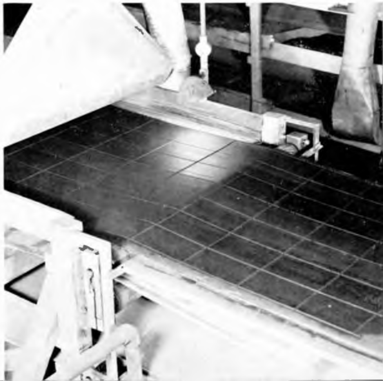
Left: The huge Banbury mixer, occupying two floors, blends all the ingredients into the final disc to master perfection. Right: Having been cut to size the plastic material moves over a conveyor belt to the room which contains the stampers. Each rectangle is the "biscuit"
