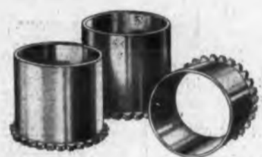
Silver Airplane Bearings made by Conn. Used in B-29 Superfortresses and many other planes using Wright Cyclone engines, including the B-17 Flying Fortress.
