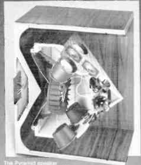
The Pyramid speaker incorporates a unique fully symmetrical folded bass horn which in turn allows the mid and hi frequency drivers to be optimally mounted for wide dispersion. The overall result is a single full range, high level, extremely efficient speaker ideally suited to discotheques.
