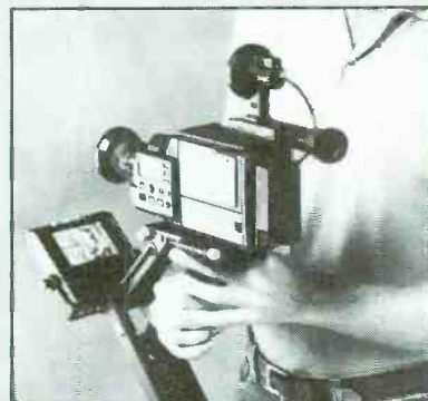
Cinema Products' Steadicam JR camcorder stabilizing system allows for never-before-achieved image steadiness.
