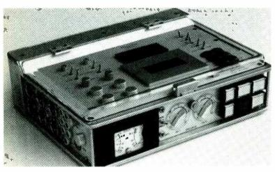
Swiss DAT. This rugged-looking portable, professional DAT machine manufactured by Stellavox is the first DAT deck from Switzerland. It offers a number of interesting features, including an incorporated mixer option for up to four microphones; a hefty 10-hour battery life; and climate-control mechanisms to handle difficult weather conditions. Contact Stellavox at 038-244400 in Neuchatel, Switzerland.
